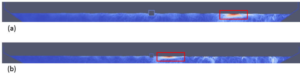
Figure 5-10 Red boxes show the area where unphysical errors appear in the NWT due to single precision inaccuracy for larger domain size of (a) L = 20 m and (b) L = 30 m.
