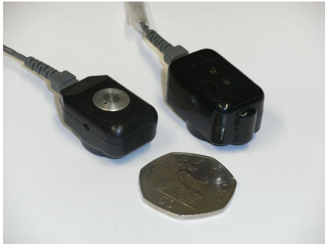
Figure 3.1 Comparison of the size and shape of the cases of the BEST (left) and B71 (right) showed next to a 50p piece.
