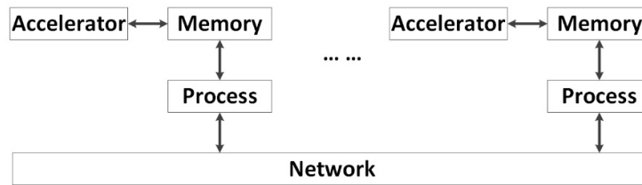
Figure 1.9 Sketch of heterogeneous programming model.
