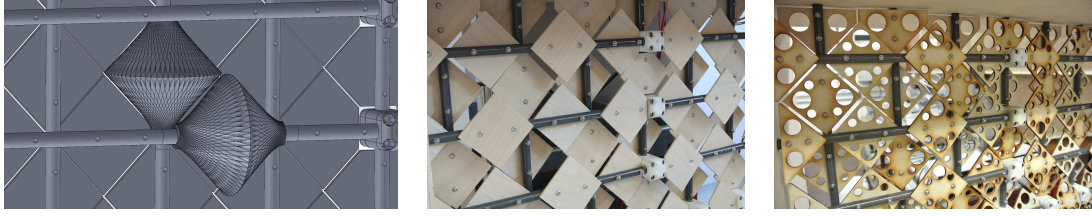
(a) CAD model (by Robert Bleischwitz) showing two representative wings in operation to test against crash. Note that the position of the non-rotating wings along the rods, i.e. non-alternating facing directions, does not reflect final configuration.
