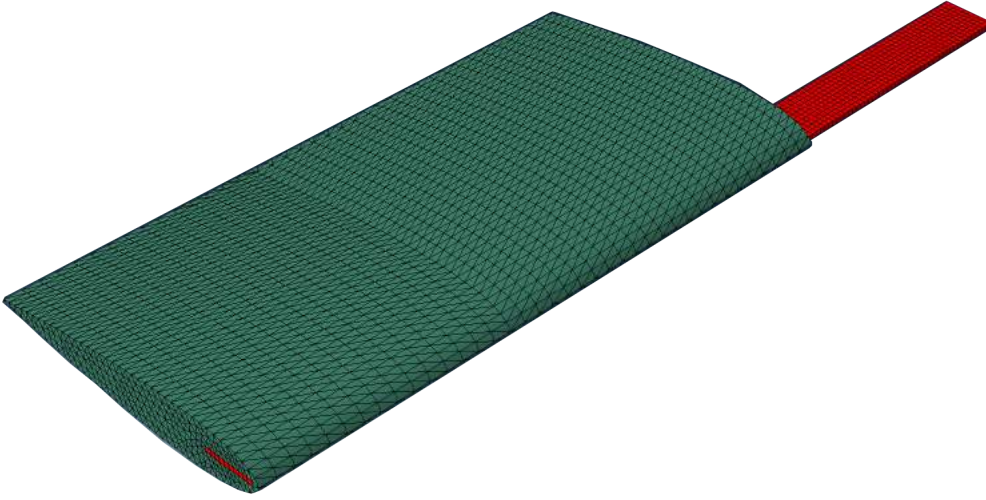
FIGURE 4.9: Aerofoil flexible structure made of PAC beam ( \phi = -30^\circ ) and full-foam aerodynamic part.
