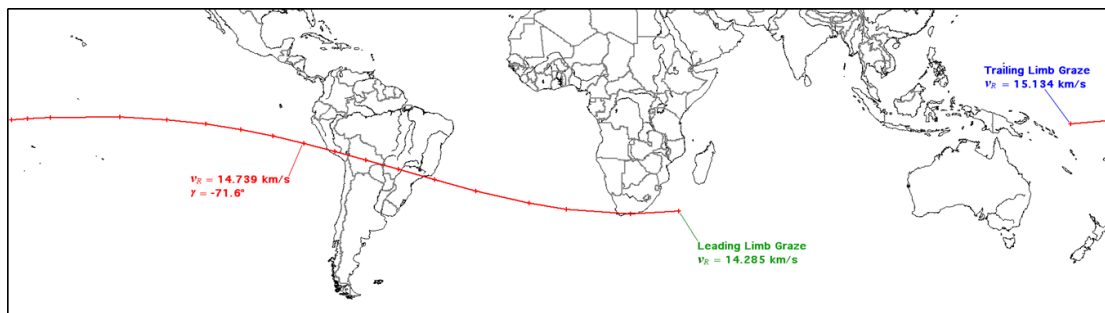
Figure 3.8: Impact line for 2011 AG5 as published by Adamo (2012). The flight path angle in the middle of the corridor is marked as -71.6^\circ and its norm corresponds to the impact angle.
