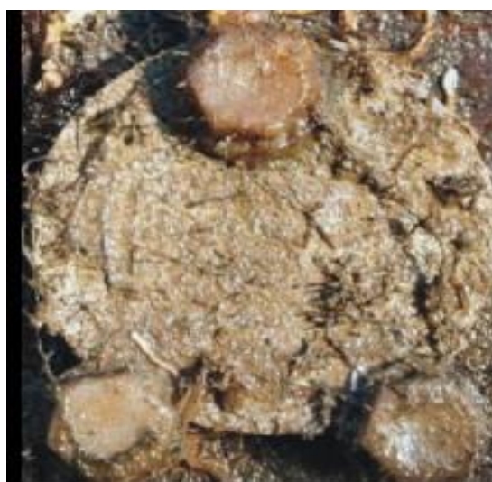
Figure 12 – Biofouling of a NAB coupled Ti disc sample immersed in seawater for 12 months at National Oceanography Center at Southampton [67].
