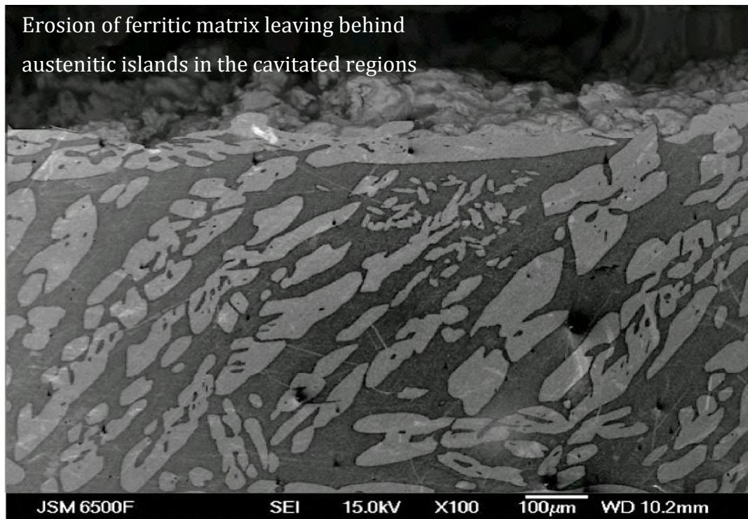
Fig. 5.19: Transverse of the DSS cavitated in 3.5% NaCl solution for 1 h.
