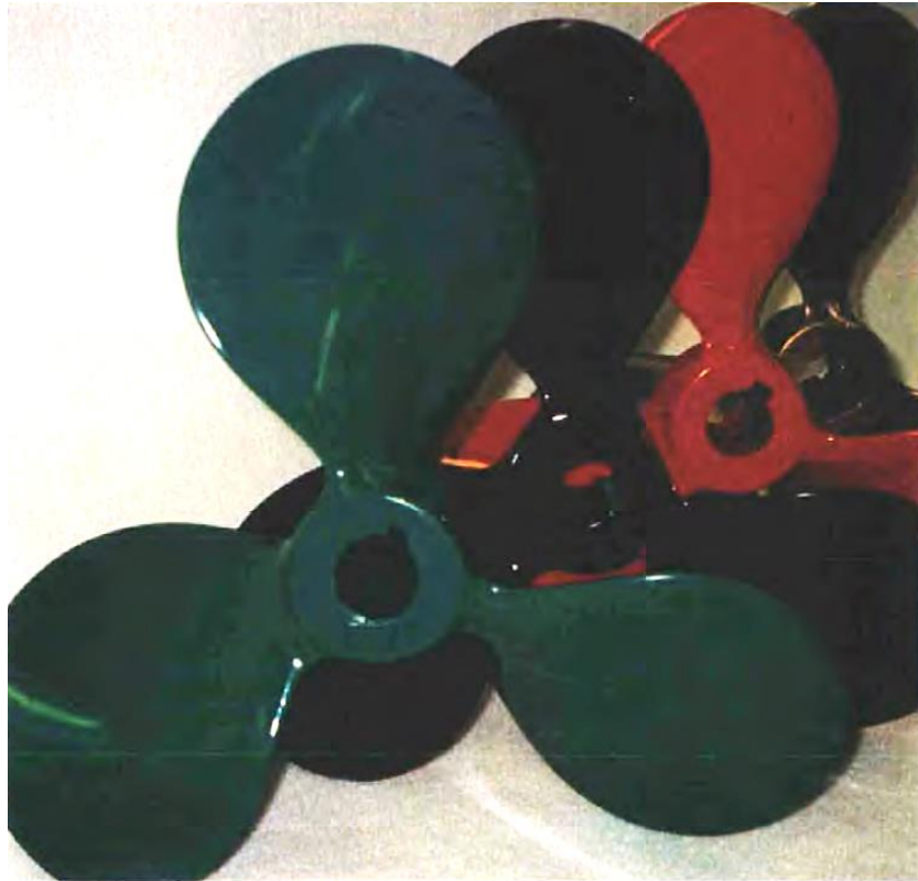
Fig 8.1: FRP propeller of diameter 305 mm painted in preparation for open water testing [248].
