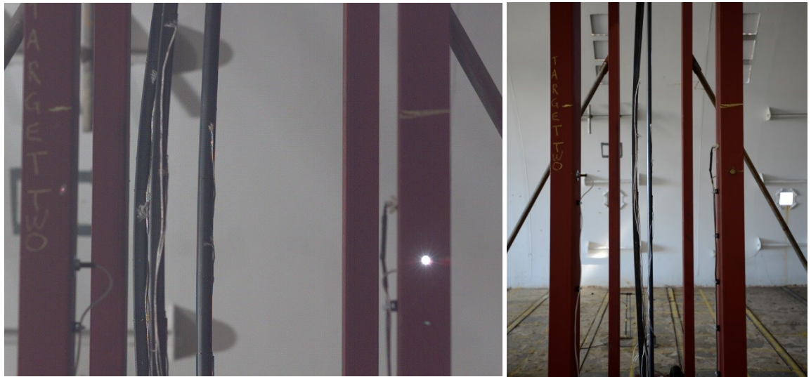
Figure 3.3.75a & b: Fifth Trial (3) Maximum (a) and Final (b) Deflected Shapes: Rig 2
