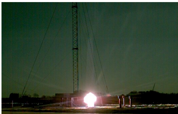
(a): Fireball at 0.81msec after Ignition
