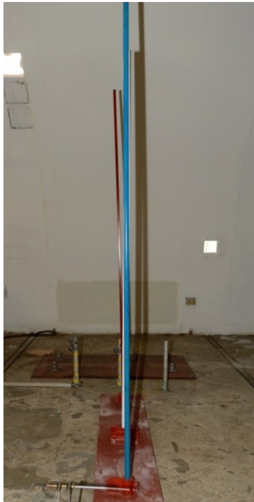
Figure 3.3.15: Post-Shot Deformation of Steel Columns in ABT
