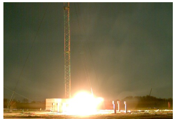
(b): Fireball at 1.0msec after Ignition
