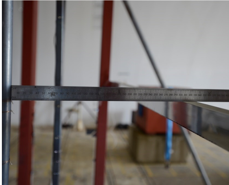
Figure 3.3.44: Post-Shot Deflection Measurement
