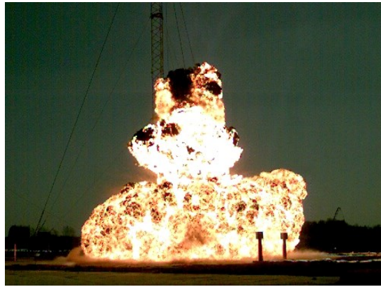
(d): Fireball at 8.2msec after Ignition
