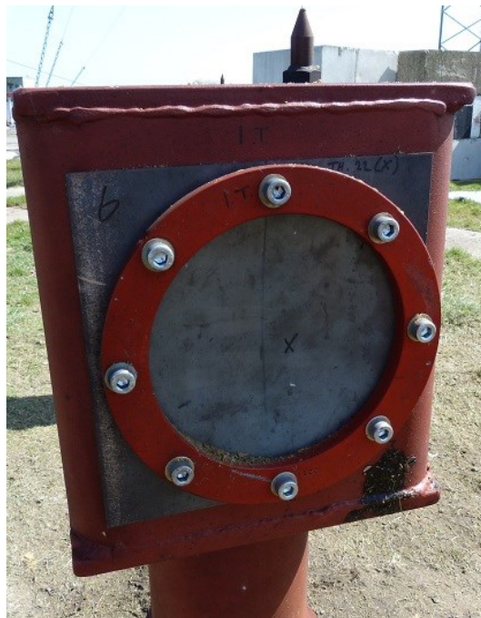
Figure 4.3.1: 2mm Steel Plate Bolted to HSB
