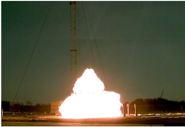
(c): Fireball at 2.2msec after Ignition
