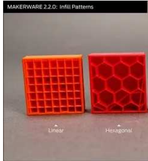
FIGURE 3.3: Two examples of conventional infills patterns that can be found in FFF-parts [12].
