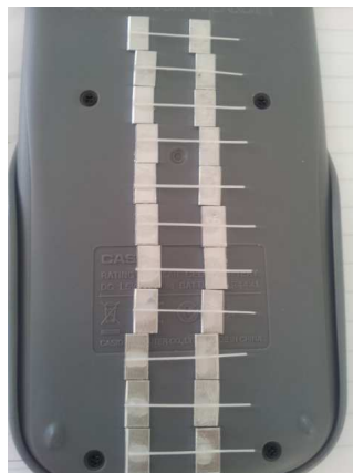
FIGURE 4.3: A photograph of single filaments glued to the clamping aluminium plates.
