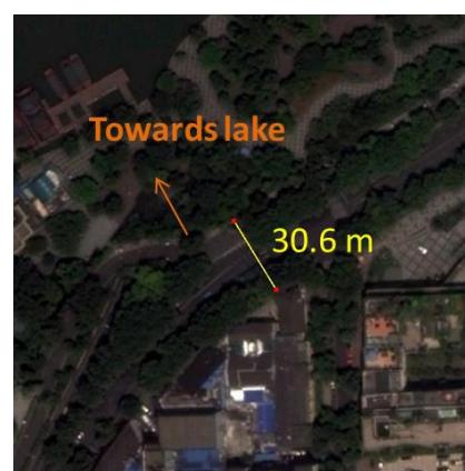
Figure 5.4. Determination of the error in street dimensions measurements based on aerial images (method used for this study) from Google Earth (Google Earth, 2013)
