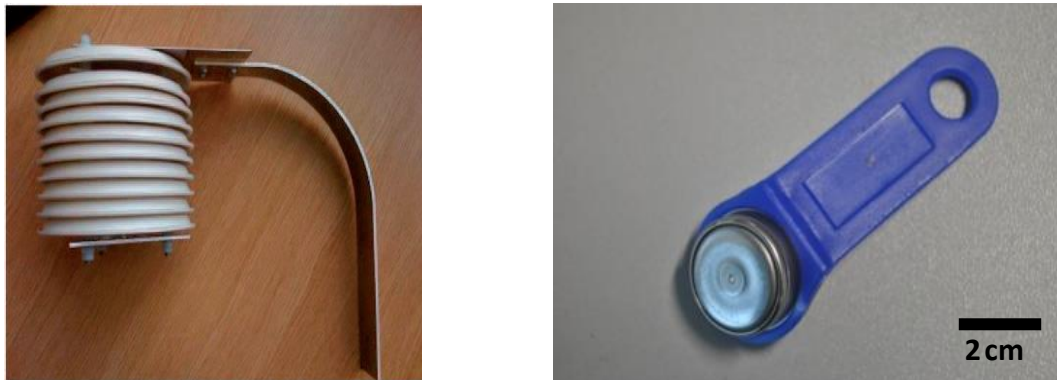
Figure 4.7. The radiation shield (Left) and the T_{\text{air}} / RH sensor (iButton©) used for the observations in China. Images Courtesy of Shen et al. (2013).
