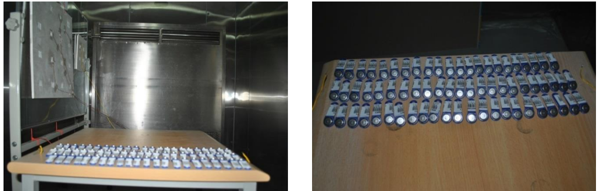
Figure 4.8. The environmental test chamber in the Centre for Sustainable Energy Technologies (CSET) at the University of Nottingham Ningbo (Left) and the sensors during the calibration (Right). Image Courtesy of Shen et al. (2013).
