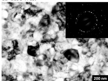
Fig.3 Bright field TEM of Ti powder consolidated by HPT (P=6 GPa and N=5 and annealed at 300 °C for 10 minutes). Inset depicts SAED.
