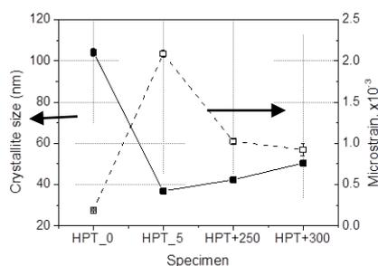
Fig.2 Crystallite size and microstrain as a function of the sample conditions: HPT\_0 corresponds to the compression at P=6 GPa, N=0, loading for 1 min; HPT\_5 corresponds to HPT straining of Ti powder at P=6 GPa, N=5; HPT+250 and HPT+300 are HPT specimens with annealing for 10 minutes at 250 and 300 °C, respectively.
