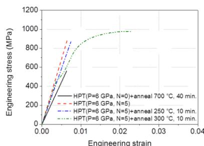
Fig.4 Engineering stress/strain plots for powder Ti subjected to HPT (RT, P=6 GPa, N=5) and additional annealing for 10 min at T=250 and T=300 °C. Black dot line is tensile plot for the samples annealed at 700 °C for 40 min. All annealing was performed in vacuum ( $10^{-3}$  torr.). Strain rate was  $10^{-3}$  s $^{-1}$ .
