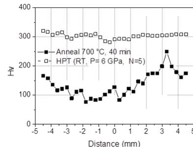
Fig.1 Microhardness, Hv across the disk diameter of Ti powder-consolidated disk annealed and HPT processed.
