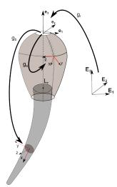
Fig. 4 illustrative scheme of the SUUV kinematics, where  $(\mathbf{E}_1, \mathbf{E}_2, \mathbf{E}_3)$  is the Euclidean fixed frame,  $(\mathbf{e}_1, \mathbf{e}_2, \mathbf{e}_3)$  represent the rigid body and is the soft bodies reference frame and  $(\mathbf{x}, \mathbf{y}, \mathbf{z})$  is the local frame for the  $\mu$ solids.
