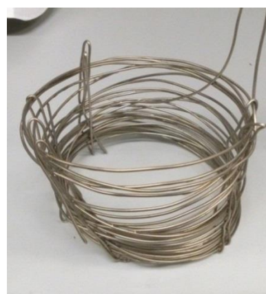
Figure 4.8: 10 mL home-made stainless steel reactor (immersed in silicon oil).
