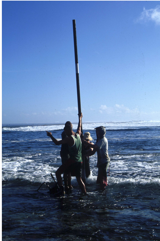
Plate 2.3 Reef drilling on Rodrigues showing drill string being manually removed from core hole to retrieve coral core.
