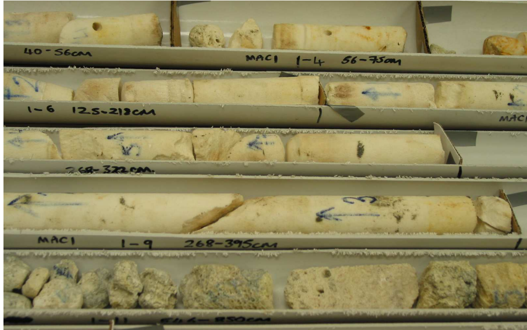
Plate 2.4 Drill core recovered from MacGillivray Reef leeward margin (Mac1). Cored material is labelled; for example, 1-9, number 1 refers to drill core name (e.g. Mac 1), number 9 refers to number of times the drill string was removed to extract coral core. The numbers and arrows labelling the coral indicate the sequence of coral pieces within each cored section. Increasing numbers indicate increasing depth from the top. Arrows indicate the orientation of the coral as it was retrieved from the core barrel. The orientation and order of the coral section retrieved assists in determining whether or not the coral was recovered in growth position, this is especially important for selecting material for radiometric dating and calculating accretion rates.
