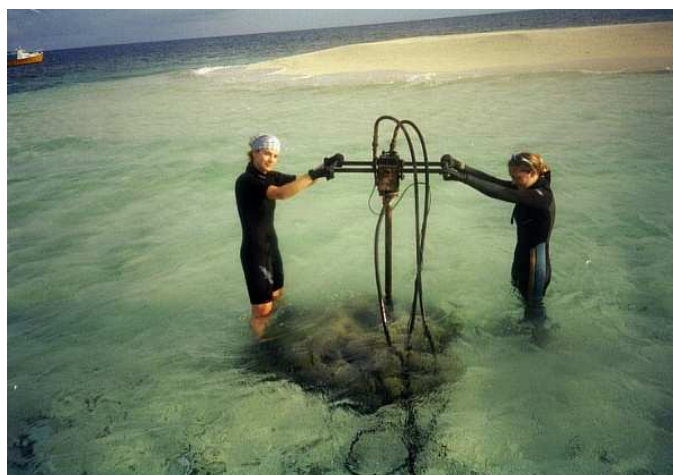
Plate 2.2 Drilling into a thrown up coral head to access the reef margin below, near the leeward sand cay on MacGillivray Reef ( 14^{\circ}39.916'S , 145^{\circ}29.310'E ). Photo taken from support dinghy harbouring generator and water pump.
