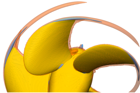
(c) Predicted cavity extent - blue ( \alpha = 0.5 ) and tip vortex - orange ( |\omega| = 1500 \text{ s}^{-1} )
