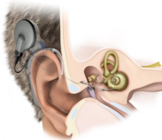
Figure 2.1 The external and internal parts of a CI. External: a microphone-processor system is worn on the ear and the transmitter is connected to it and magnetically attached to the internal receiver-stimulator. Internal: the receiver-stimulation system placed under the skin and the electrode array placed within the cochlea. Photo: MED-EL.
