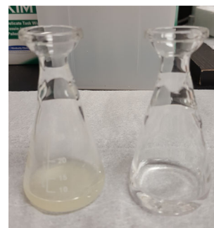
Fig. 5 Comparison of combustion water obtained using the Parr 1121 (left) and HBO 2 (right)
