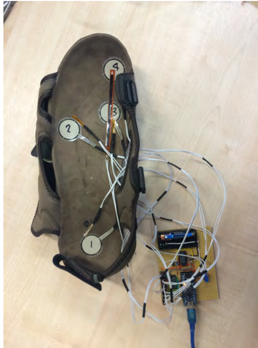
Figure 3.6: Analogue circuit prototype board, for the investigation of force, temperature and forefoot flexure
