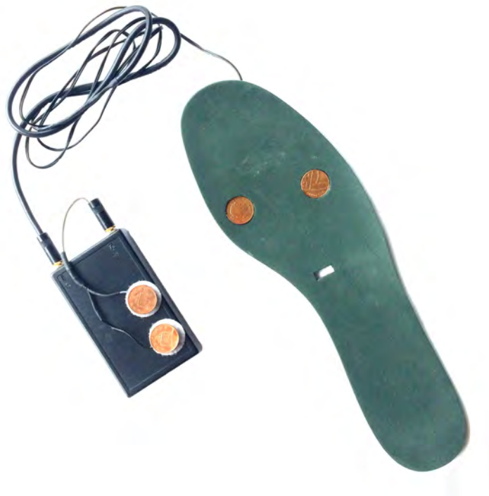
Figure 4.1: Foot to hand GSR measurement device
