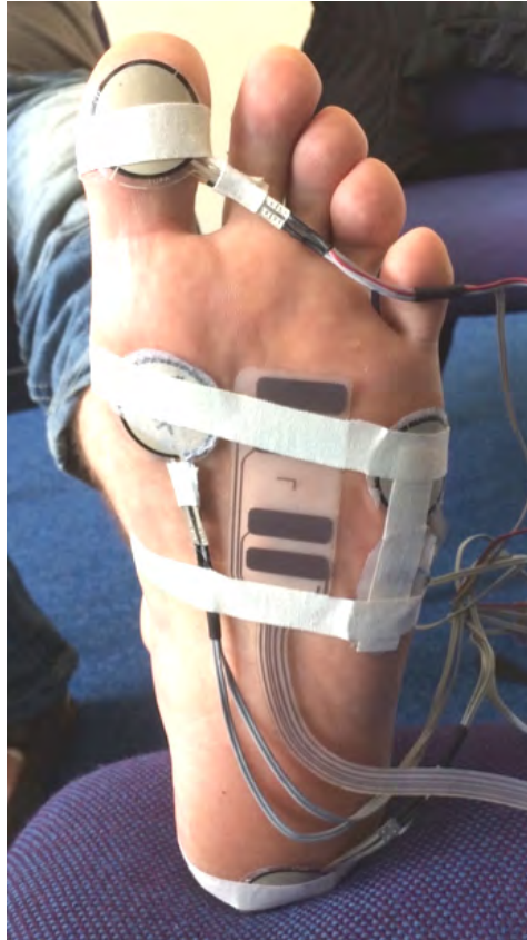
Figure 5.8: Sensors fitted directly to the foot
