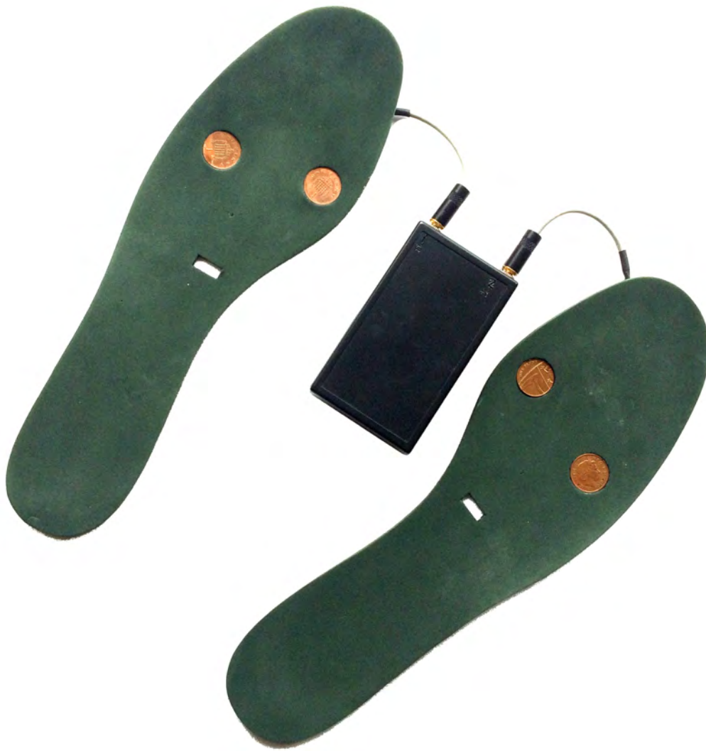
Figure 4.6: Intra pedal GSR measurement device
