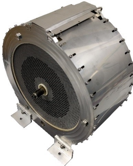
Figure 5.2: ITT thruster having a discharge chamber diameter of 17 cm, as designed for the LEOSWEEP mission.
