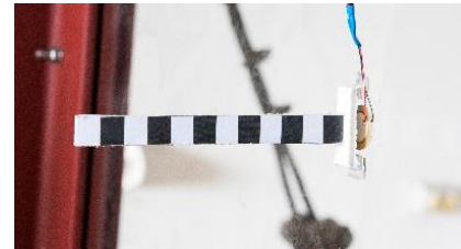
Figure 5. Deflection gauge used to track central deflection.
