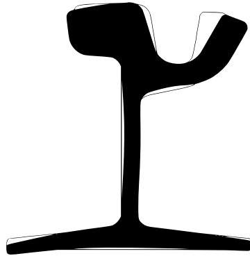
Figure 3.9: Head flapping of 60R1 rail (3109 Hz - \xi = 0 rad/m)
