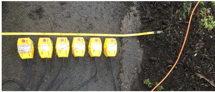
Figure 7.6: MISW experimental set-up configuration for the asphalt test site, with the discontinuity outside the array of sensors (in this case the edge of the road pavement).
