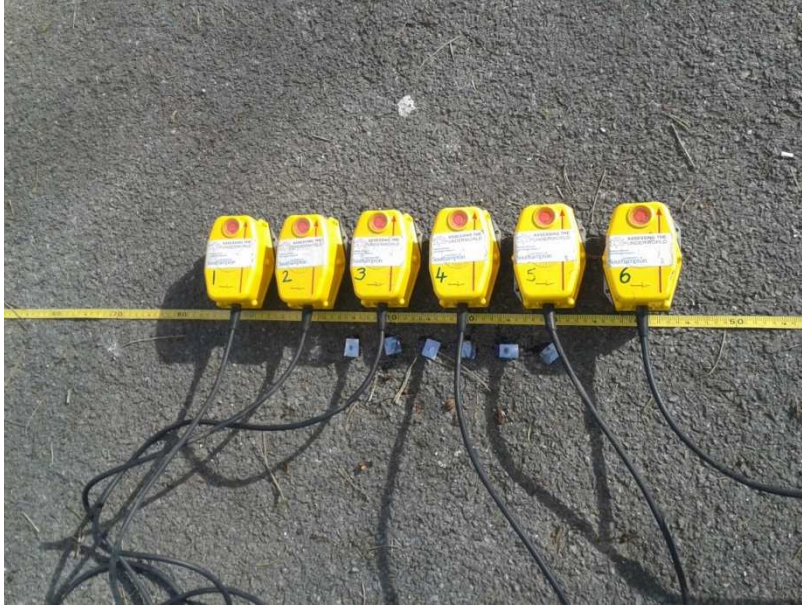
Figure 5.33: Experimental set-up for the dispersion measurement of asphalt.
