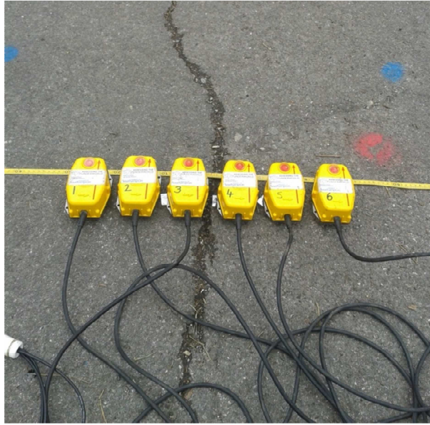
Figure 7.10: MISW experimental set-up configuration for the asphalt test site, with the discontinuity located in the middle of the array of sensors.
