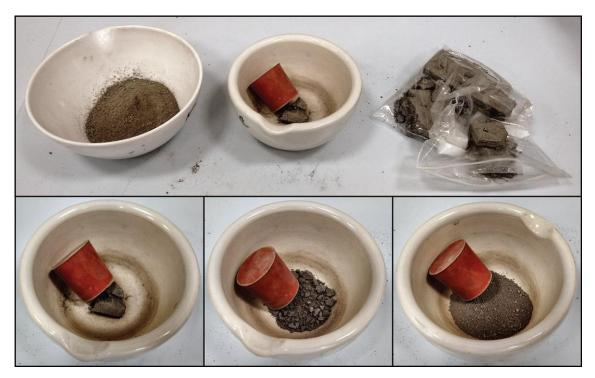
Figure 14: post-test disaggregation procedure. Top right shows the sample after drying overnight in the oven, top left shows the final disaggregated sample, top centre and bottom row shows the progression in disaggregation.
