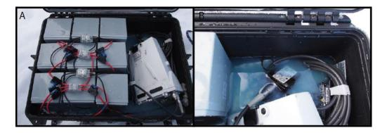
Figure 75: A) Water intrusion into GEF4's power supply after 12 months. B) Damage to the power controller.
