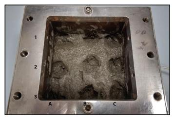
Figure 20: Shear box filled in pre-test state, after samples for moisture and LOI have been removed.
