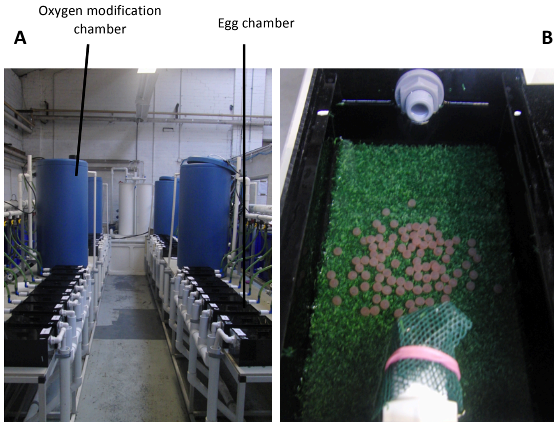
Figure 2.3. Photograph of (A) experimental set-up showing large blue oxygen modification chambers with smaller black perspex egg chambers and (B) egg chambers lined with artificial grass and containing fertilised Atlantic salmon eggs.
