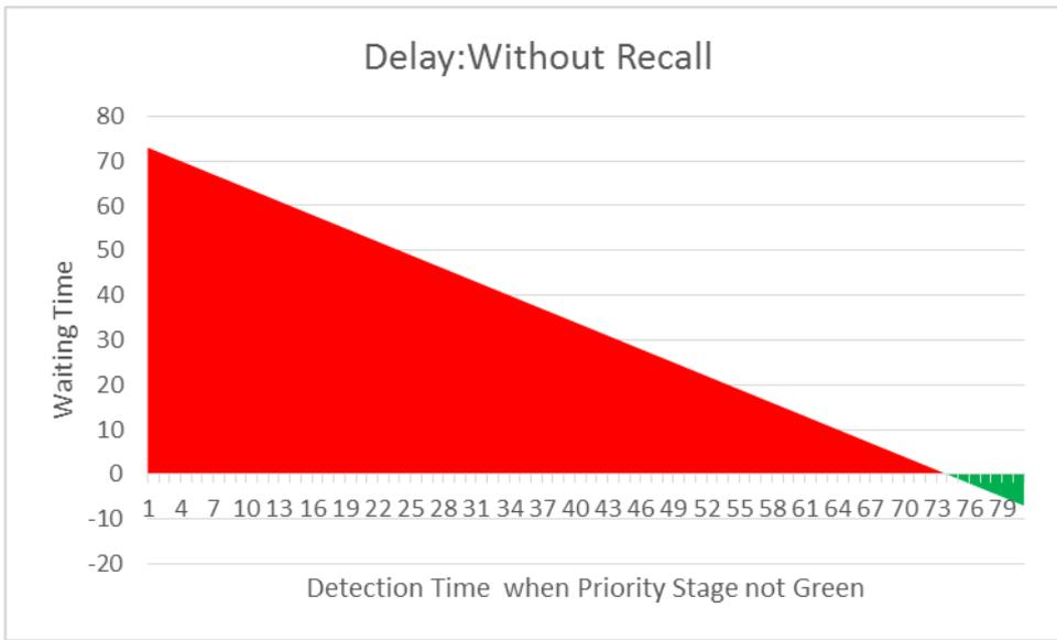
Figure 4.30: Delay to buses without recall with time of detection
