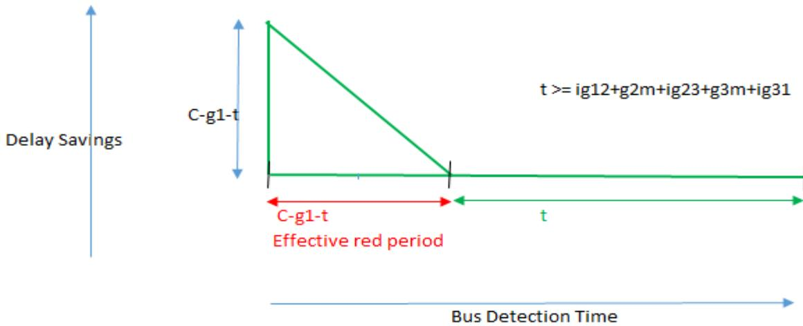
**Figure 4.22:** Bus delay savings due to each recall with time of detection ( $t \geq ig_{12}+g_{2m}+ig_{23}+g_{3m}+ig_{31}$ )
