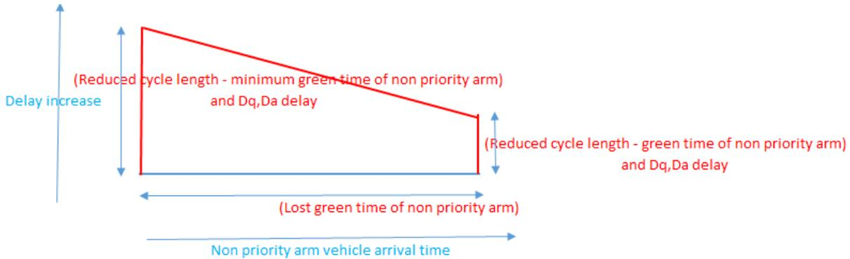
**Figure 4.36:** Delay increase to non priority arm due to recall (Condition 1)
