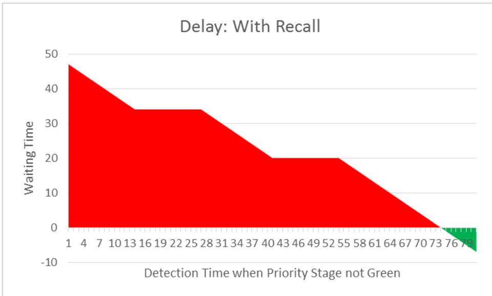
Figure 4.31: Delay to buses due to each recall with time of detection
