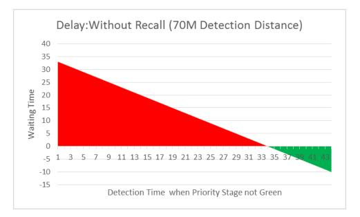
Figure 3.6: More buses needed recall due to short detection distance
