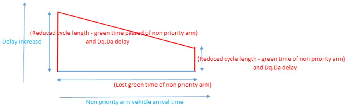
**Figure 4.37:** Delay increase to non priority arm due to recall (Condition 2)
