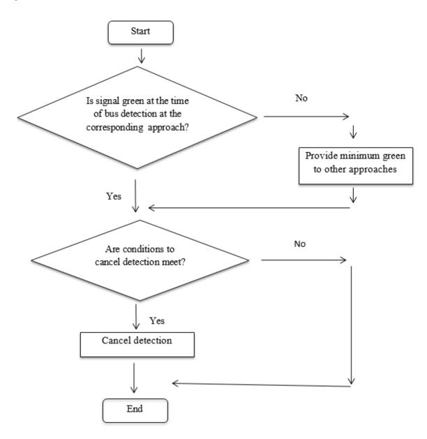
Figure 6.14: Bus priority module for recall
