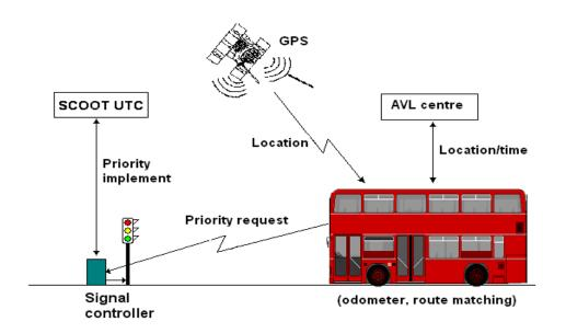
Figure 2.1: Simple representation of bus priority at traffic signals using iBus
