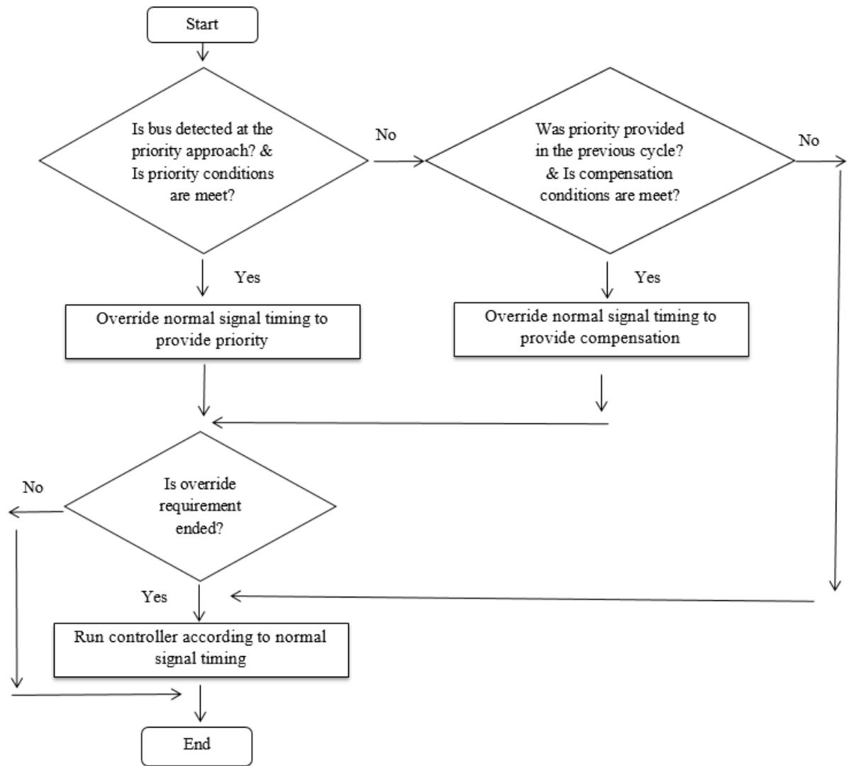
**Figure 6.4:** Signal controller's basic working methodology
