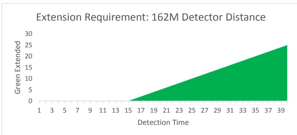
**Figure 3.5:** Buses provided longer extension due to longer detection distance
