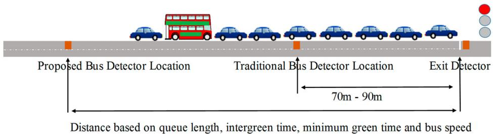
Figure 5. (Colour online) Limitations when bus detector is located close to the junction.
