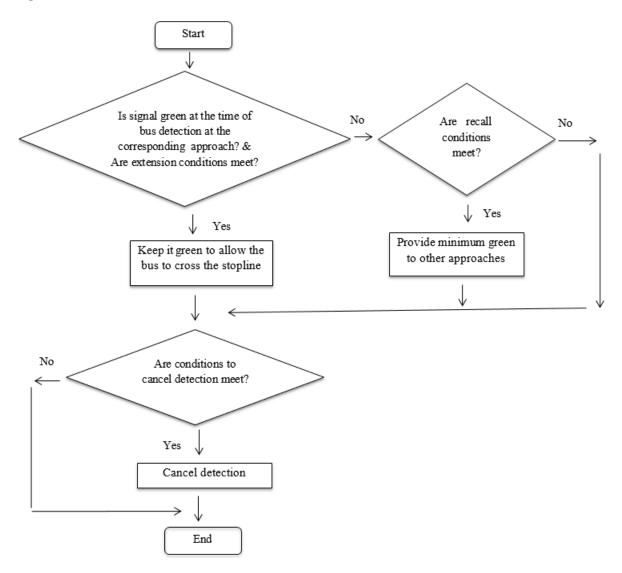
Figure 6.15: Bus priority module for extension & recall (together)
