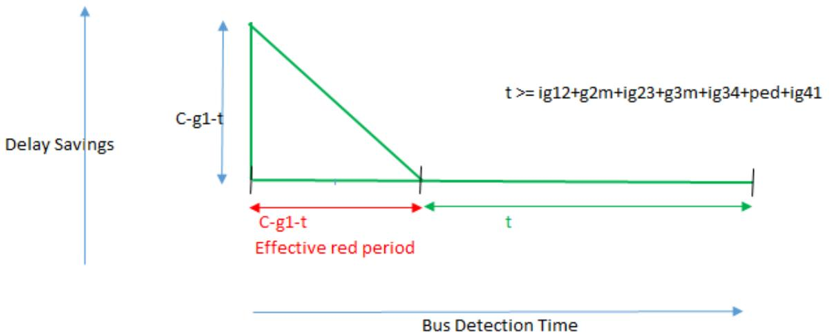
**Figure 4.29:** Bus delay saving due to each recall with time of detection ( $t \geq ig_{12}+g_{2m}+ig_{23}+g_{3m}+ig_{34}+ped+ig_{41}$ )
