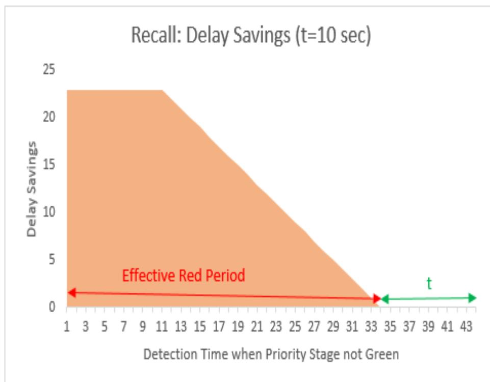
**Figure 3.8:** Effective red period and delay savings for  $t = 10$  sec
