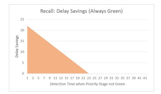
Figure 4.47: Delay savings to buses by recall for always green bus with time of detection (two traffic stage junction)
