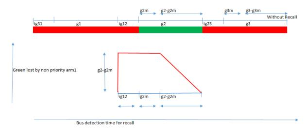
Figure 4.40: Lost green time due to each recall at non priority arm1
