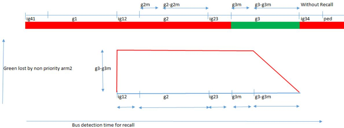
**Figure 4.43:** Lost green time due to each recall at non priority arm2
