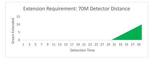
Figure 3.3: Buses provided short extension due to short detection distance
