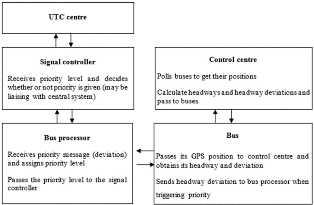
**Figure 2.2:** Functional diagram of main components of differential priority in iBus
