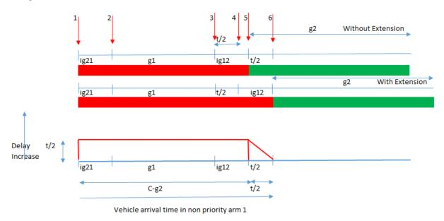
Figure 4.5: Delay increase due to green extension to non priority arm1 (two stage)
