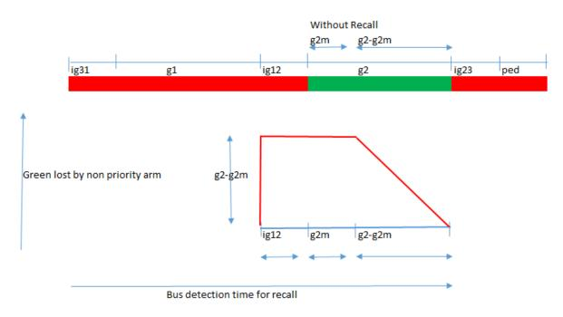
Figure 4.39: Lost green time on the non priority arm due to each recall
