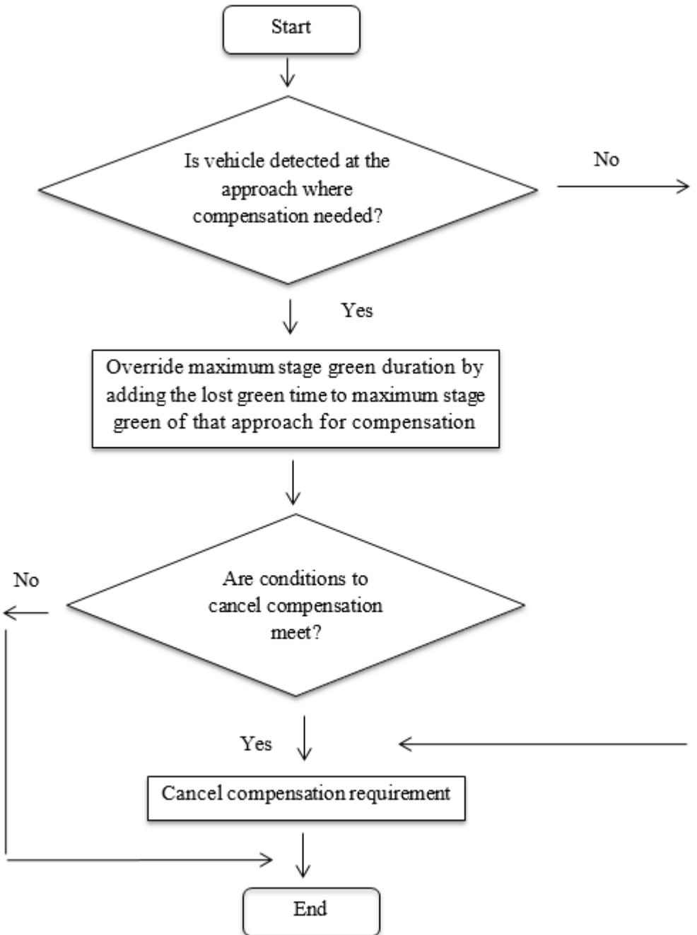
Figure 6.21: Stage compensation module
