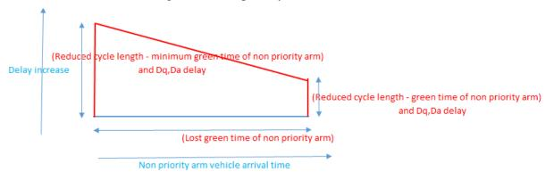
Figure 4.36: Delay increase to non priority arm due to recall (Condition 1)
