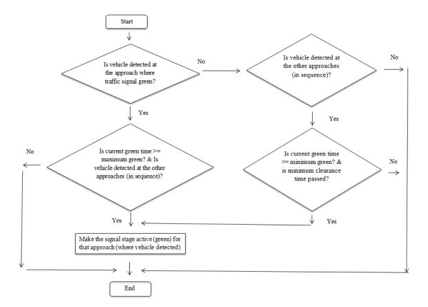
Figure 6.5: Isolated VA signal controller (normal setting)
