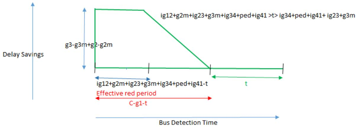
**Figure 4.28:** Bus delay saving by each recall with time of detection ( $ig_{12}+g_{2m}+ig_{23}+g_{3m}+ig_{34}+ped+ig_{41} > t > ig_{34}+ped+ig_{41}+ig_{23}+g_{3m}$ )
