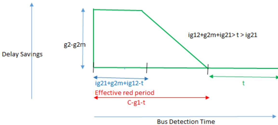
**Figure 4.8:** Bus delay saving due to each recall with time of detection ( $ig12+g2m+ig21 > t > ig21$ )
