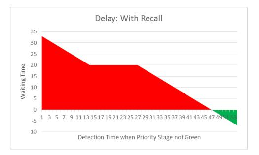
Figure 4.17: Delay to buses due to each recall with time of detection
