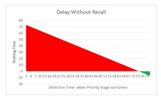
Figure 4.30 below illustrates the delay to buses without recall with time of detection.
