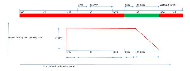
Figure 4.43: Lost green time due to each recall at non priority arm2
