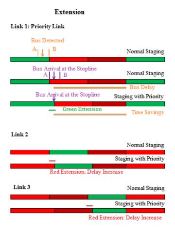
Figure 6.11: Phase diagram without and with extension
