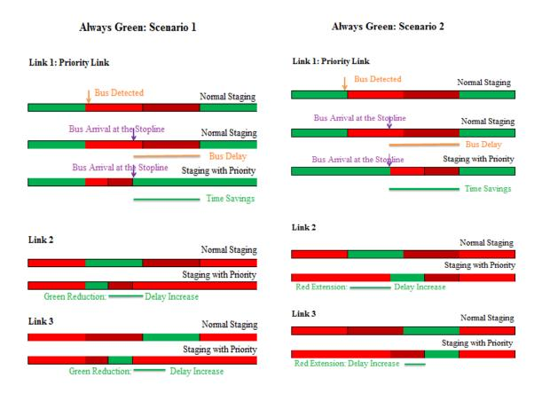
Figure 6.18: Phase diagram without and with 'always green bus'
