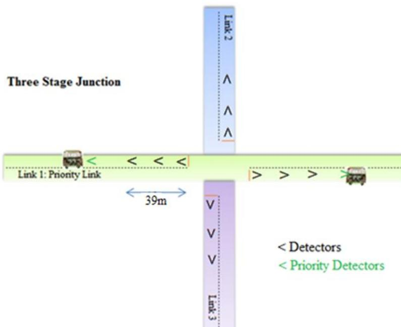
**Figure 6.10:** Typical three stage cross junction
