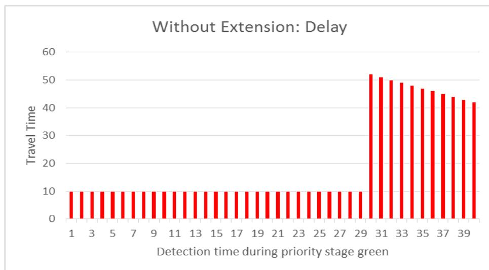
**Figure 4.2:** Delay without extension
