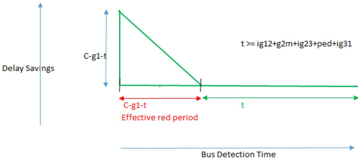
**Figure 4.15:** Bus delay saving due to each recall with time of detection ( $t \geq ig12+g2m+ig23+ped+ig31$ )
