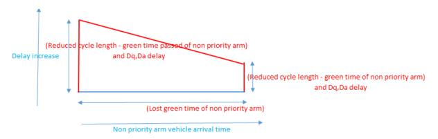
Figure 4.37: Delay increase to non priority arm due to recall (Condition 2)
