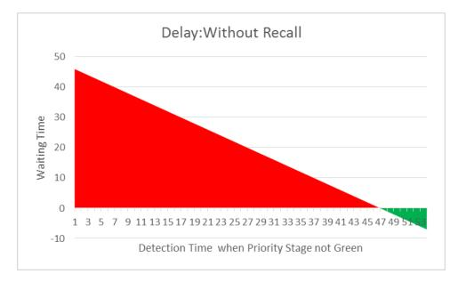
Figure 4.16: Delay to buses without recall with time of detection
