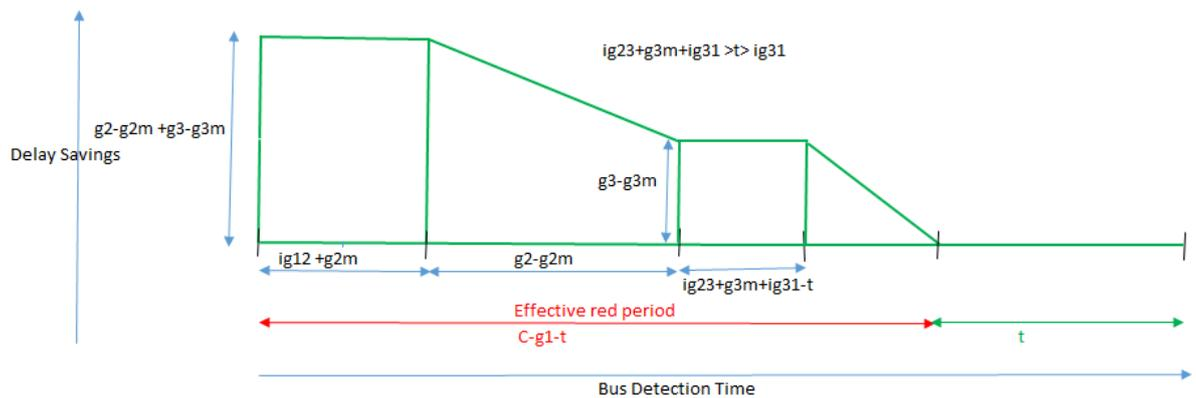
**Figure 4.20:** Bus delay savings due to each recall with time of detection ( $ig_{23} + g_{3m} + ig_{31} > t > ig_{31}$ )
