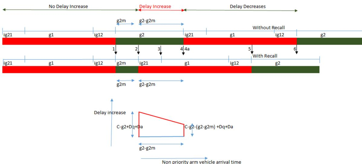
Figure 4.33: Delay increase to non priority arm due to recall
