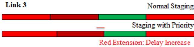
**Figure 6.11:** Phase diagram without and with extension
