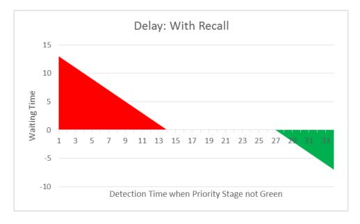
Figure 4.11 below illustrates the delay to buses due to a recall with time of detection.
