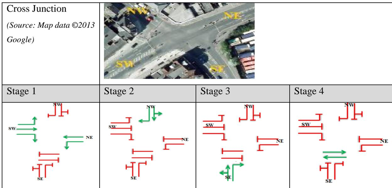
Figure 5.5: Cross junction stage diagram
