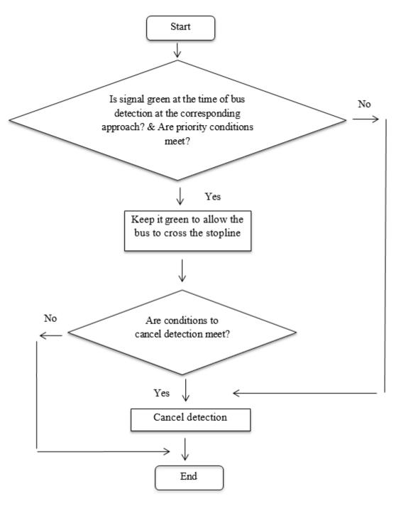
Figure 6.12: Bus priority module for extension
