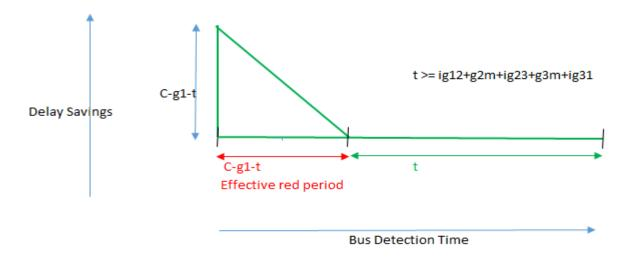
Figure 4.22: Bus delay savings due to each recall with time of detection (t > = ig12+g2m+ig23+g3m+ig31)
