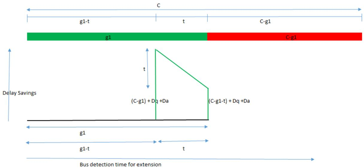
**Figure 4.1:** Delay savings by extension with time of detection
