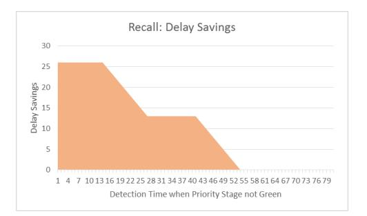
Figure 4.32: Delay savings to buses by recall with time of detection
