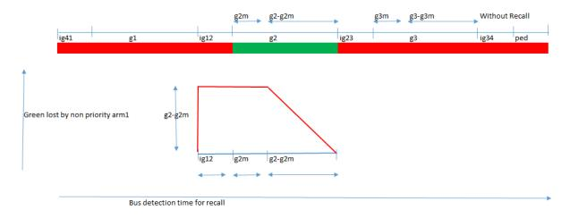
Figure 4.42: Lost green time due to each recall at non priority arm1
