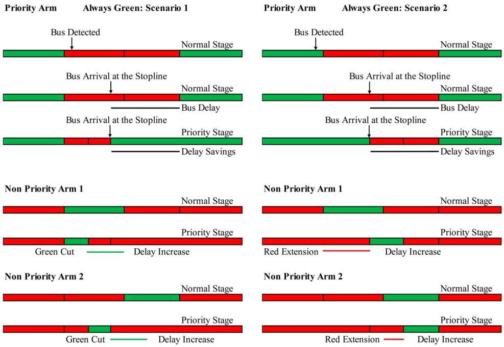
Figure 6. (Colour online) Phase diagram without and with always green for bus.
