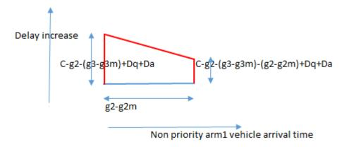
Figure 4.34: Delay increase to non priority arm1 due to recall
