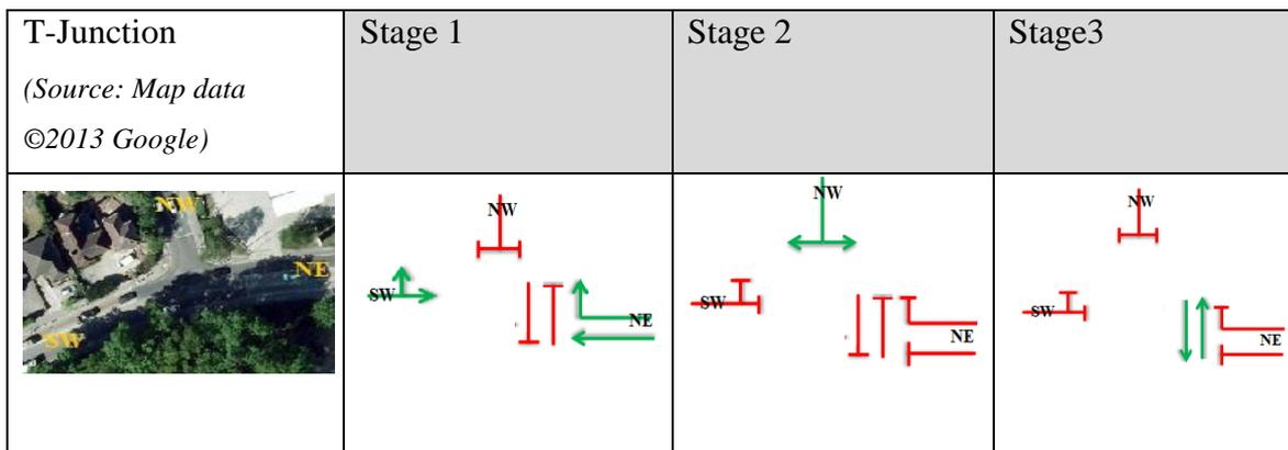
**Figure 5.7:** T-junction signal stage diagram
