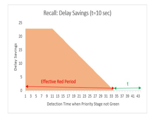
Figure 3.8: Effective red period and delay savings for t =10 sec
