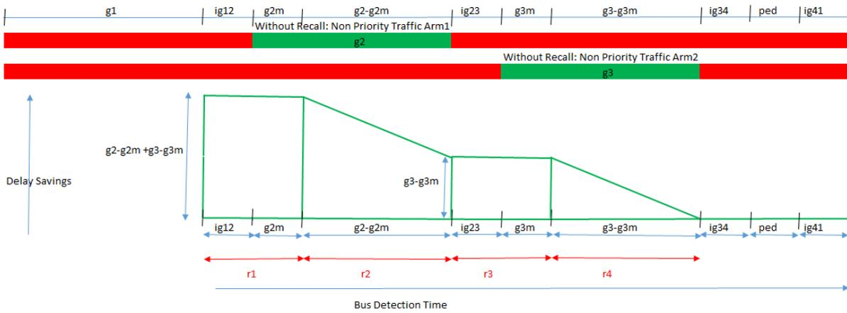
Effective red period =  $r_1 + r_2 + r_3 + r_4 = C - g_1 - ig_{34} - ped - ig_{41}$  (when  $ig_{34} + ped + ig_{41} \geq t$ )
