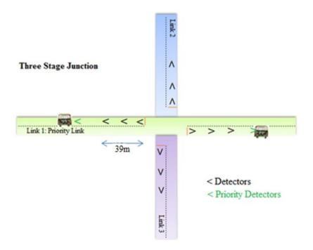
Figure 6.10: Typical three stage cross junction
