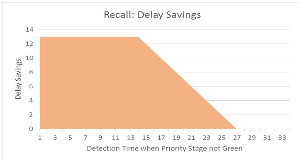
**Figure 4.12:** Delay savings to buses by recall with time of detection
