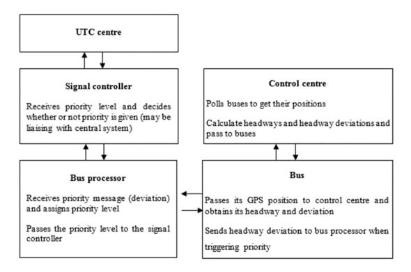
Figure 2.2: Functional diagram of main components of differential priority in iBus
