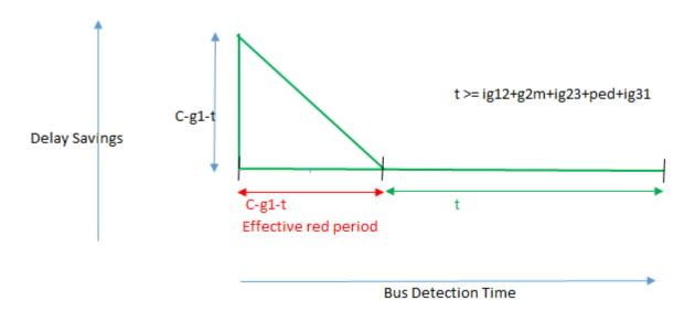
Figure 4.15: Bus delay saving due to each recall with time of detection (t >= ig12+g2m+ig23+ped+ig31)
