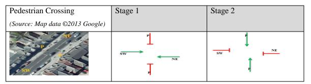
Figure 5.6: Pedestrian crossing stage diagram
