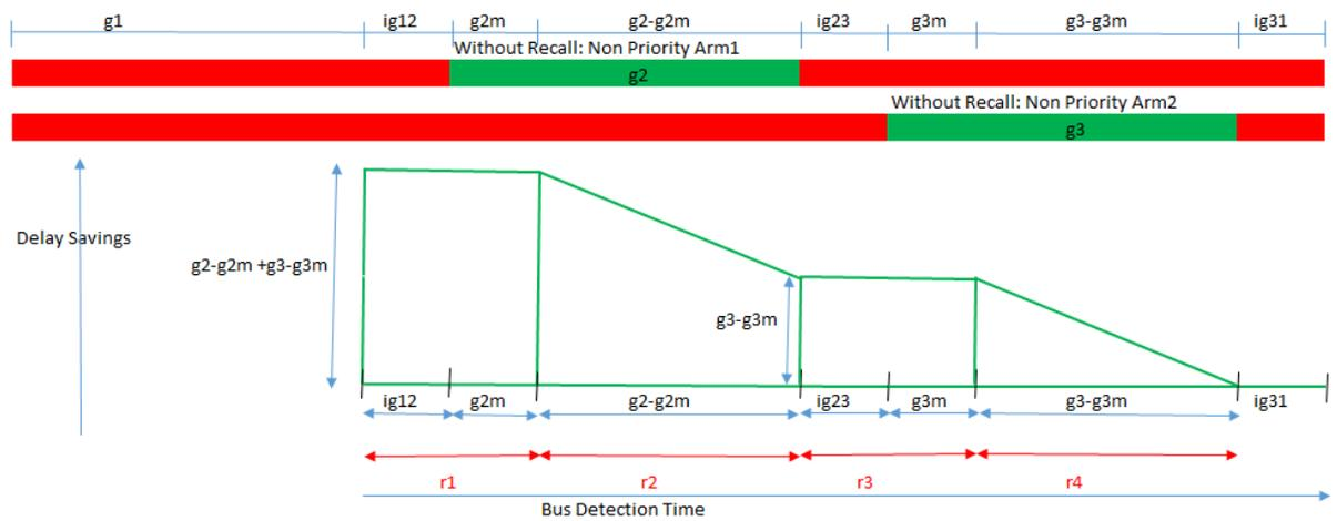
$$\text{Effective red period} = r_1 + r_2 + r_3 + r_4 = C - g_1 - ig_{31} \quad (\text{when } ig_{31} \geq t)$$
