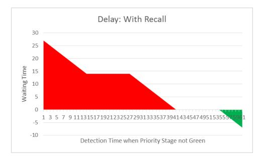
Figure 4.24: Delay to buses due to each recall with time of detection
