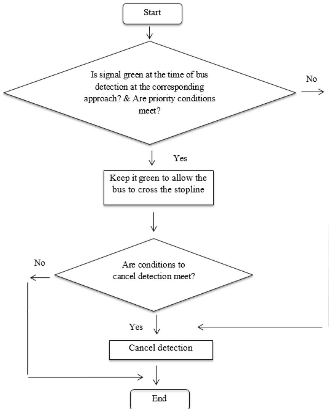
**Figure 6.12:** Bus priority module for extension
