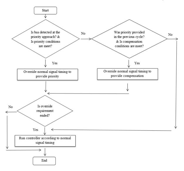
Figure 6.4: Signal controller's basic working methodology
