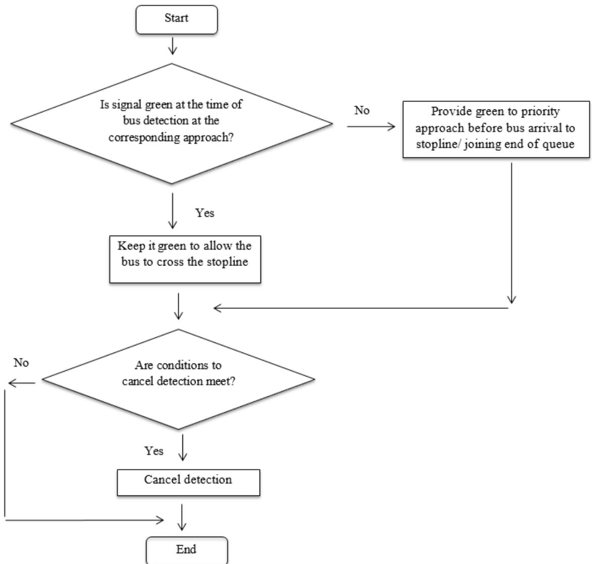
**Figure 6.19:** Bus priority module for ‘always green bus’
