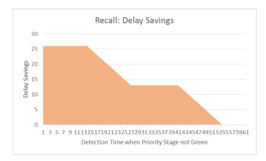
Figure 4.25: Delay savings to buses due to each recall with time of detection
