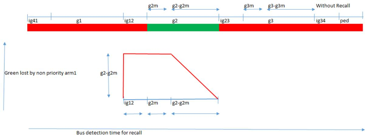
**Figure 4.42:** Lost green time due to each recall at non priority arm1
