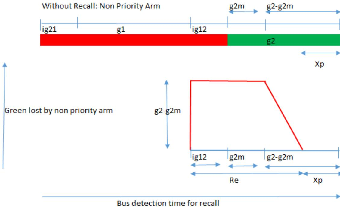
Figure 4.48: Green loss by non priority arm due to recall for always green bus (two traffic stage junction)
