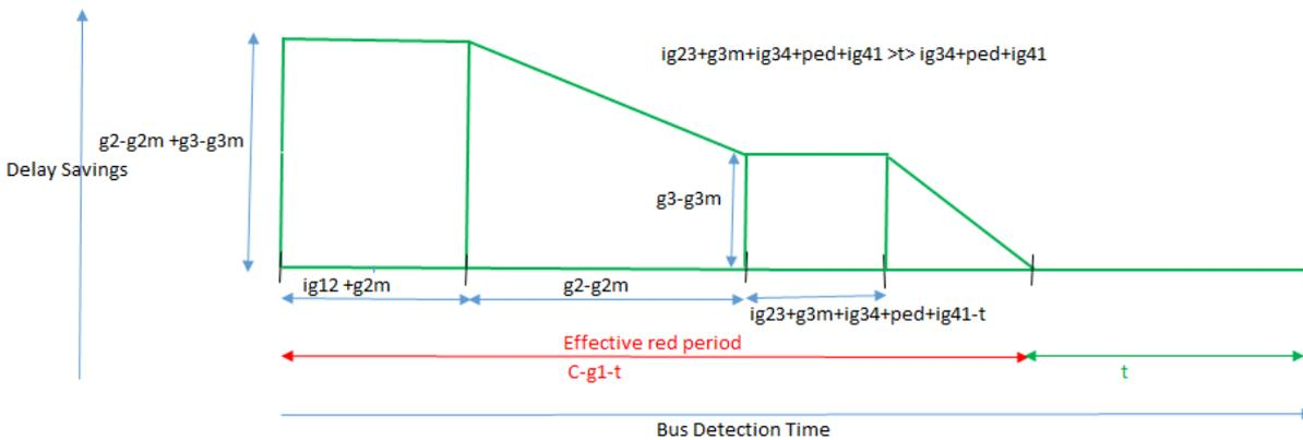
Figure 4.27: Bus delay saving due to each recall with time of detection ( $ig_{23} + g_{3m} + ig_{34} + ped + ig_{41} > t > ig_{34} + ped + ig_{41}$ )
