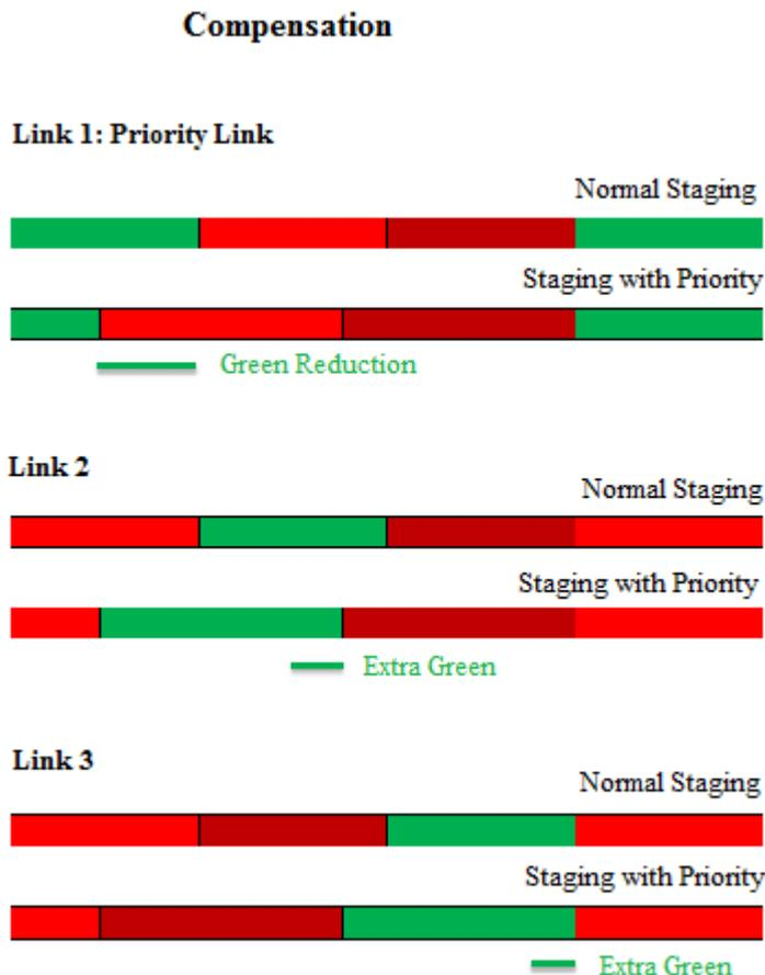
**Figure 6.20:** Phase diagram without and with compensation
