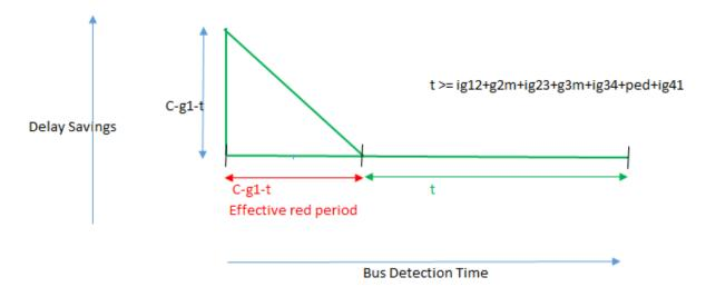
Figure 4.29: Bus delay saving due to each recall with time of detection (t>= ig12+g2m+ig23+g3m+ig34+ped+ig41)
