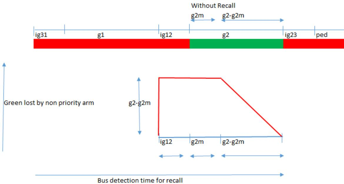
**Figure 4.39:** Lost green time on the non priority arm due to each recall
