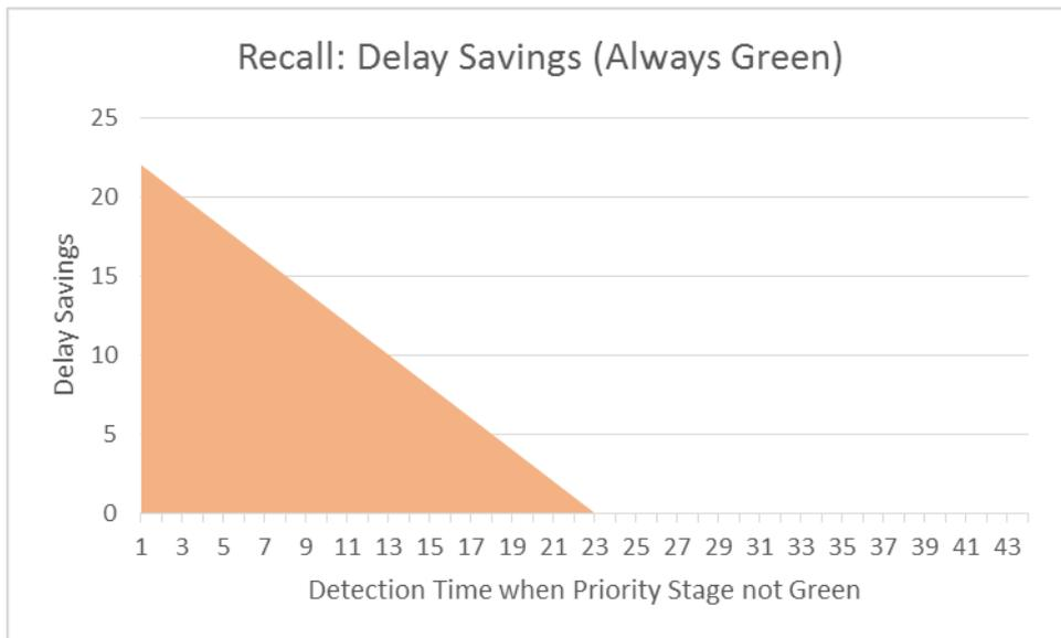
**Figure 4.47:** Delay savings to buses by recall for always green bus with time of detection (two traffic stage junction)
