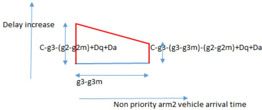
**Figure 4.35:** Delay increase to non priority arm2 due to recall
