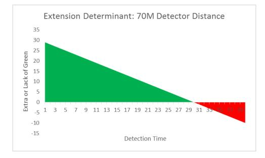
Figure 3.2: Buses needed short extension due to short detection distance
