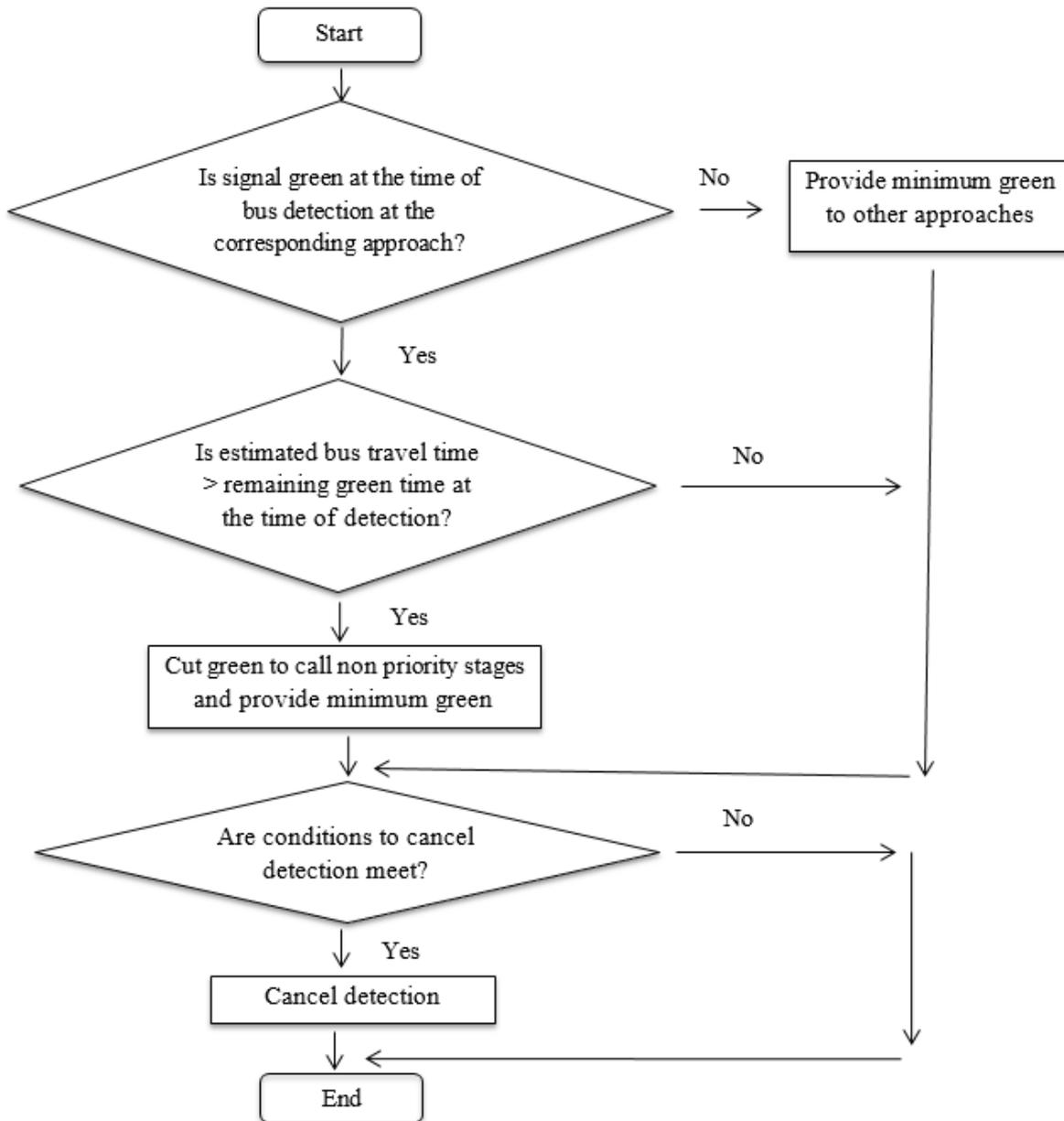
**Figure 6.17:** Bus priority module for cut & recall
