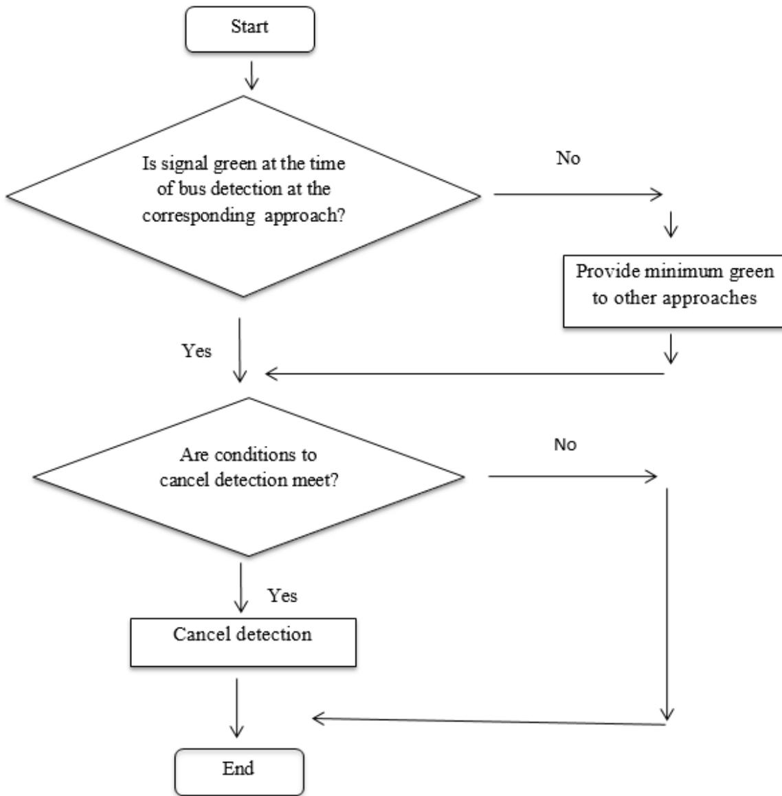
**Figure 6.14:** Bus priority module for recall
