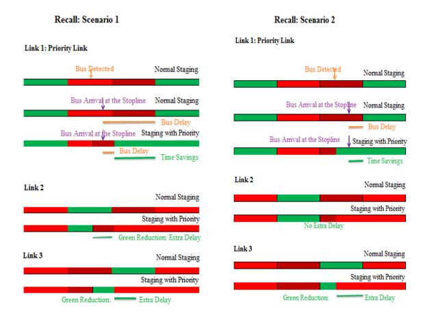
Figure 6.13: Phase diagram without and with recall
