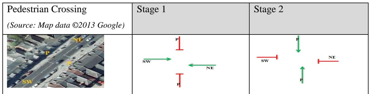
**Figure 5.6:** Pedestrian crossing stage diagram**Table 5.12:** Pedestrian crossing signal stage details
