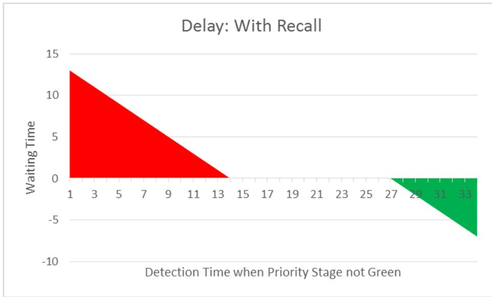
**Figure 4.11:** Delay to buses due to a recall with time of detection
