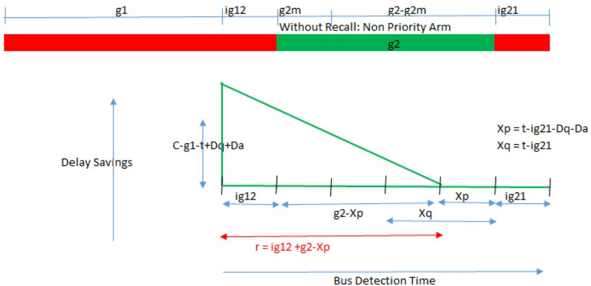
**Figure 4.44:** Bus delay saving due to each recall for always green bus with time of bus detection (two traffic stage junction)
