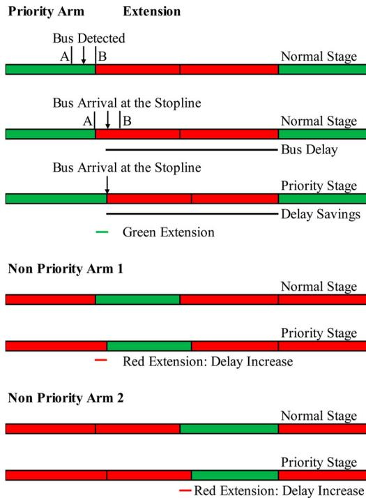
**Figure 3.** (Colour online) Phase diagram without and with extension.
