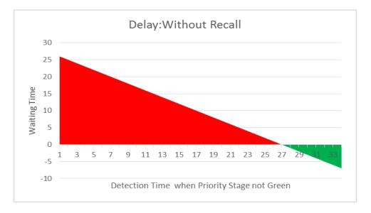
Figure 4.10: Delay to buses without recall with time of detection
