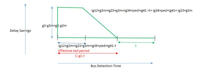
Figure 4.28: Bus delay saving by each recall with time of detection (ig12+g2m+ig23+g3m+ig34+ped+ig41 > t > ig34+ped+ig41+ig23+g3m)
