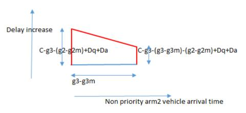
Figure 4.35: Delay increase to non priority arm2 due to recall
