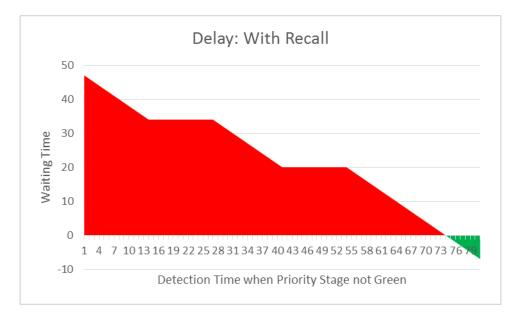
Figure 4.31: Delay to buses due to each recall with time of detection
