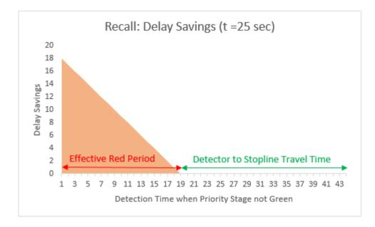
Figure 3.9: Effective red period and delay savings for t =25 sec
