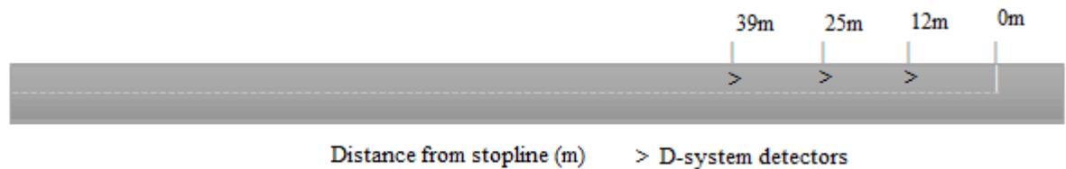
**Figure 6.6:** Location of D-system detectors
