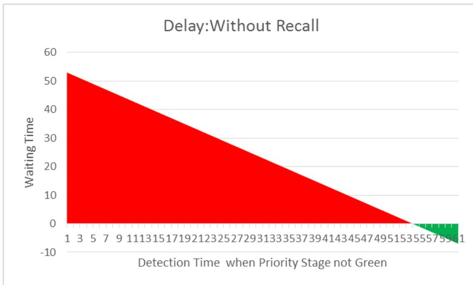
**Figure 4.23:** Delay to buses without recall with time of detection
