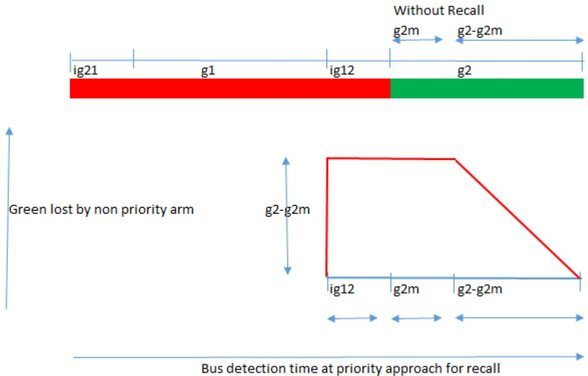
**Figure 4.38:** Lost green time due to each recall at non priority arm
