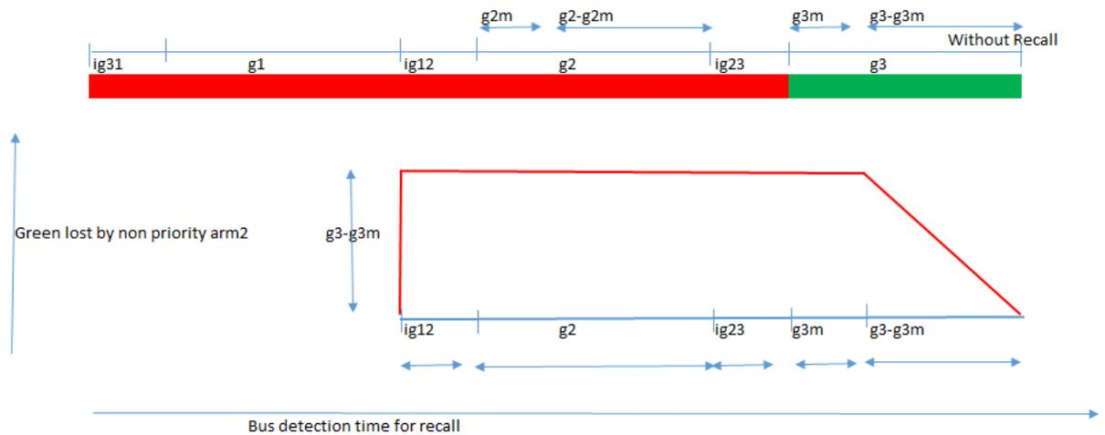
**Figure 4.41:** Lost green time due to each recall at non priority arm2
