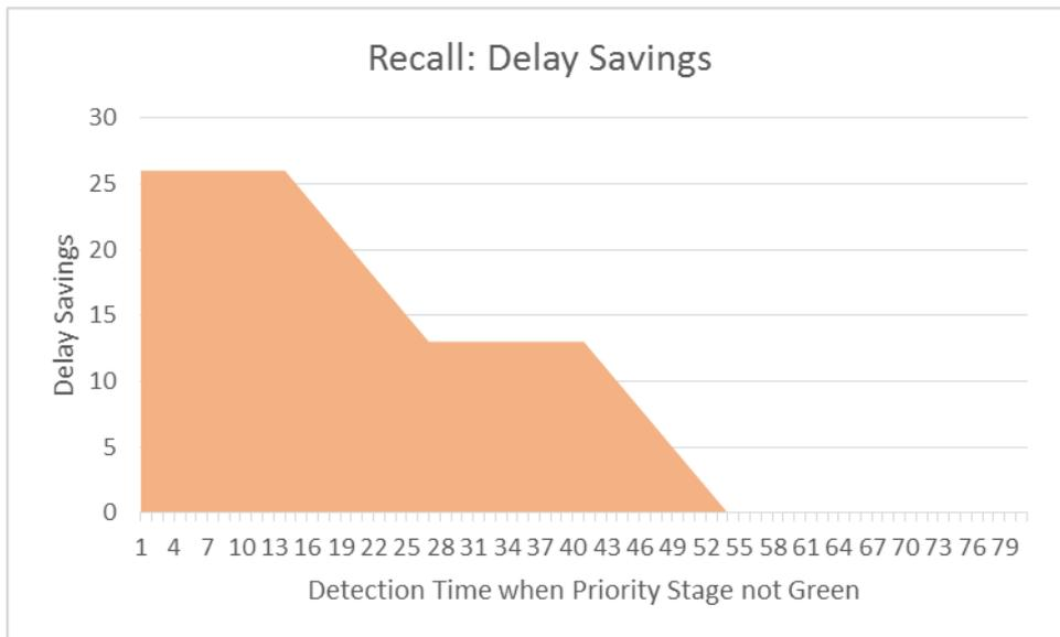
**Figure 4.32:** Delay savings to buses by recall with time of detection
