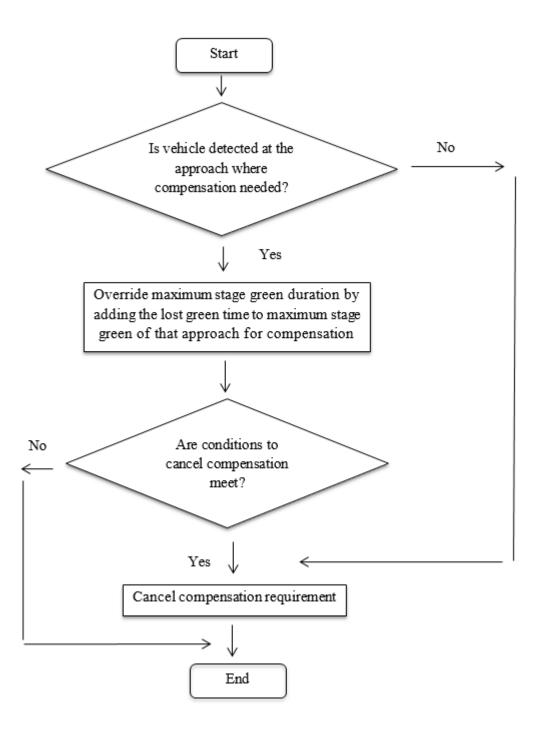
Figure 6.21: Stage compensation module
