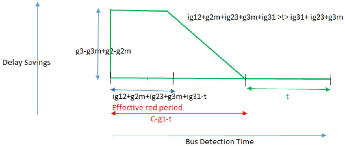
**Figure 4.21:** Bus delay savings due to each recall with time of detection ( $ig_{12}+g_{2m}+ig_{23}+g_{3m}+ig_{31} > t > ig_{31}+ig_{23}+ig_{3m}$ )
