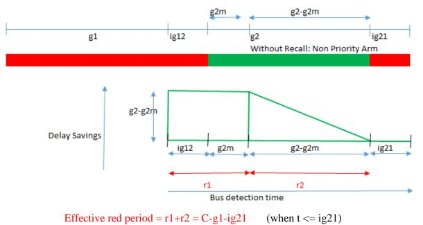
**Figure 4.7:** Bus delay saving due to each recall with time of detection ( $t \le ig21$ )
