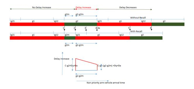
Figure 4.33: Delay increase to non priority arm due to recall
