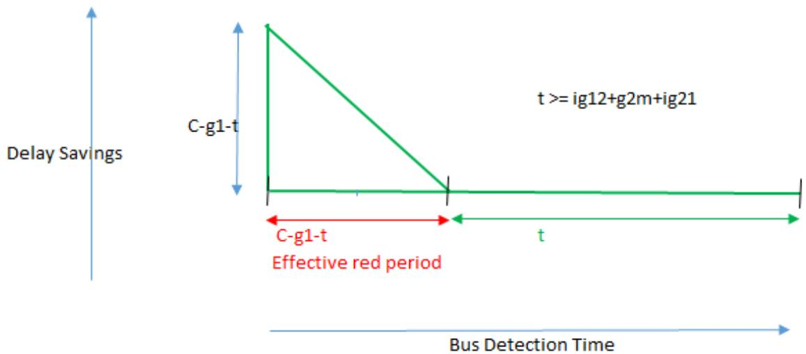
**Figure 4.9:** Bus delay saving due to each recall with time of detection ( $t \geq ig12+g2m+ig21$ )
