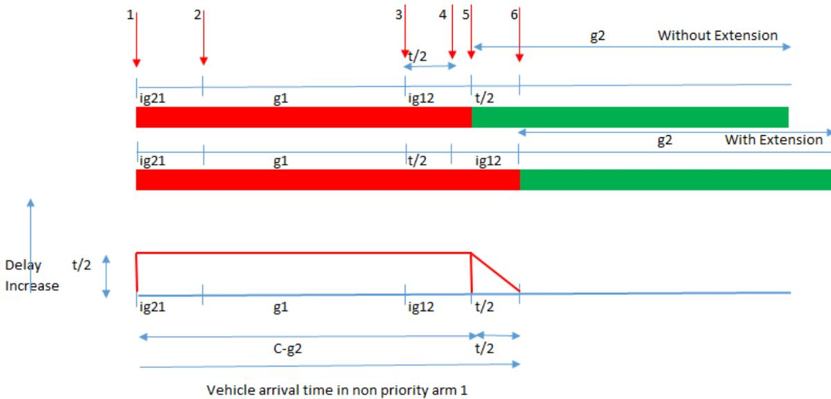
**Figure 4.5:** Delay increase due to green extension to non priority arm 1 (two stage)
