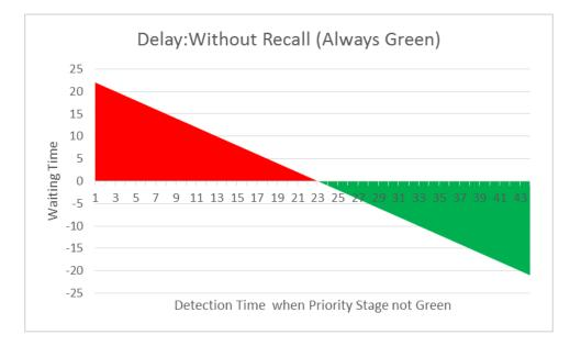
Figure 4.45: Delay to buses without recall for always green bus with time of detection (two traffic stage junction)
