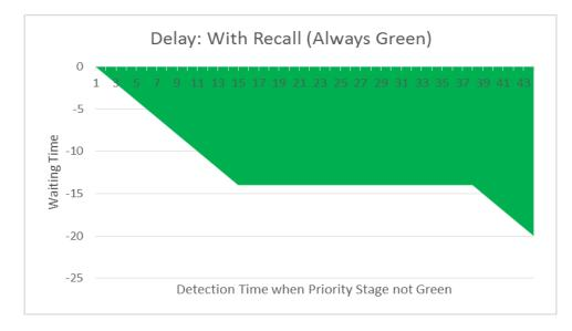
Figure 4.46: Delay to buses with recall for always green bus with time of detection (two traffic stage junction)
