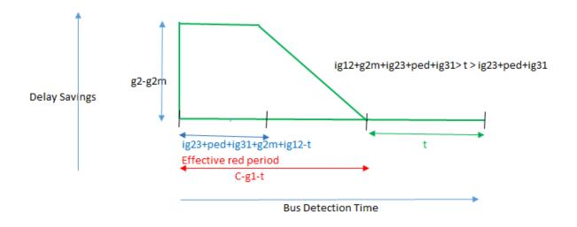
Figure 4.14: Bus delay savings due to each recall with time of detection (ig12+g2m+ig23+ped+ig31 > t > ig23+ped+ig31)
