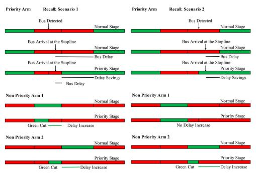
Figure 4. (Colour online) Phase diagram without and with recall.
