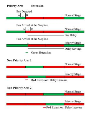
Figure 3. (Colour online) Phase diagram without and with extension.
