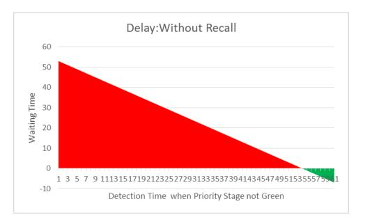
Figure 4.23 below illustrates the delay to buses without recall with time of detection.
