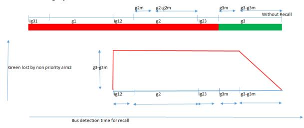
Figure 4.41: Lost green time due to each recall at non priority arm2
