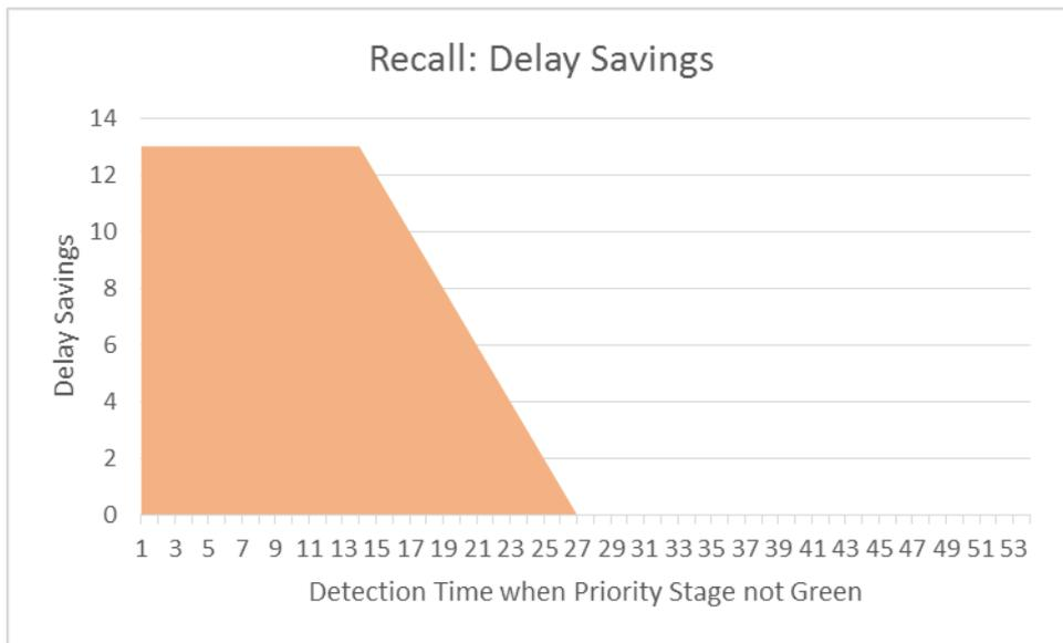
**Figure 4.18:** Delay savings to buses due to each recall with time of detection
