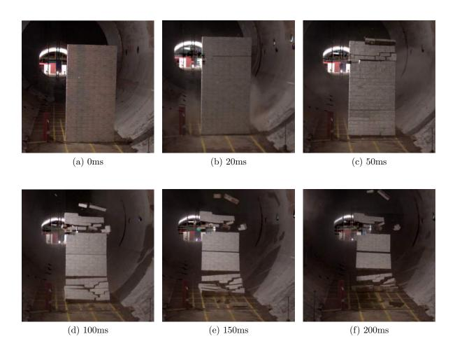
Figure 4.35: High speed photography (from the upstream perspective) of the breakage of structure BWL1A
