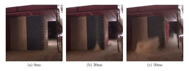
Figure 4.62: High speed photography (from the rear perspective) of the blast clearing around structure BWL2D and vortex production
