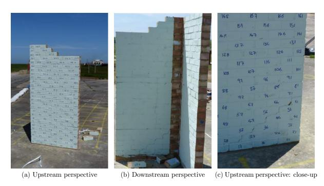
Figure 4.33: Post-shot photographs of structure WR2E
