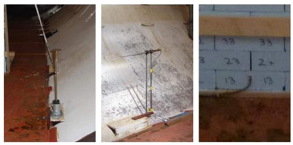
(a) Endveco-8510 (static) pressure (b) Kulite-20D (dynamic) pressure (c) Kulite-LQ125 (reflective) prestransducer transducer sure transducer at base
