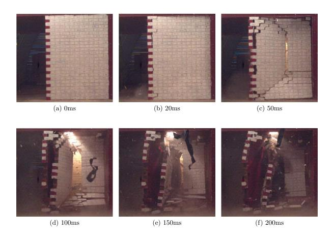
Figure 4.45: High speed photography (from the upstream perspective) of the breakage of structure BWL1C
