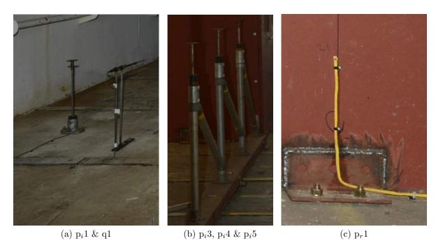
Figure 3.24: Sample set of the fixed static, dynamic and reflected pressure gauges used for the BWL series
