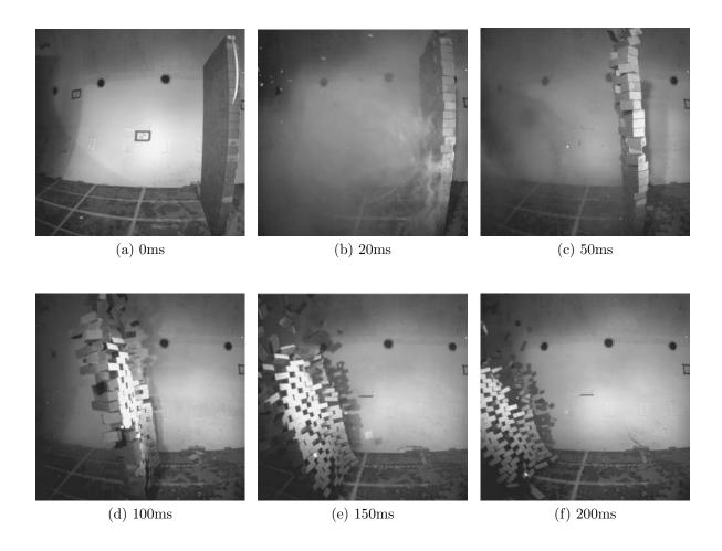
Figure 4.3: High speed photography (from the side perspective) of the breakage of structure MW1
