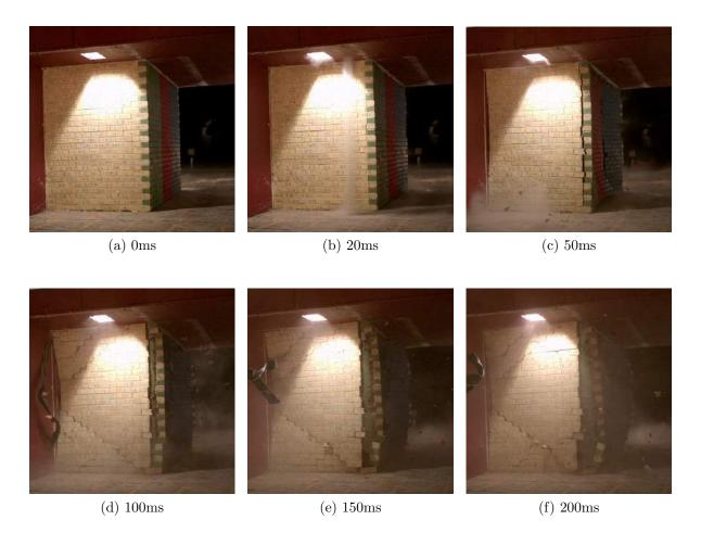
Figure 4.77: High speed photography (from the downstream perspective) of the breakage of structure BWL3C
