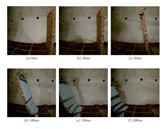
Figure 4.9: High speed photography (from the side perspective) of the breakage of structure MW2
