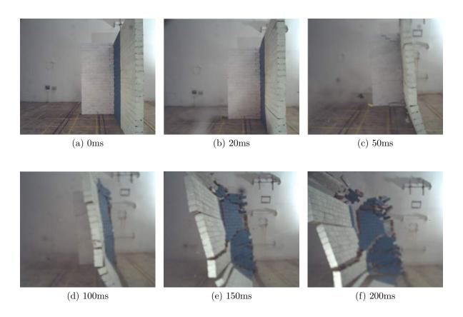
Figure 4.41: High speed photography (from the side perspective) of the breakage of structure BWL1B
