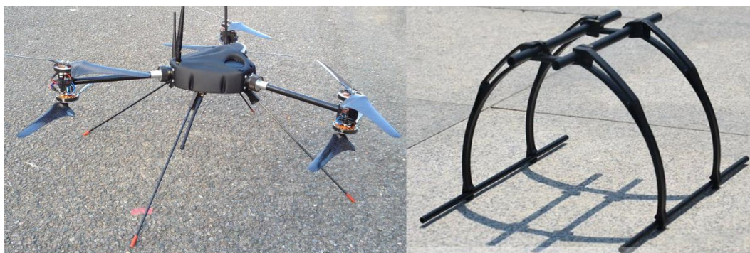
Figure 3.9 - Landing gear types. (Left) multi point, (Right) skids.
