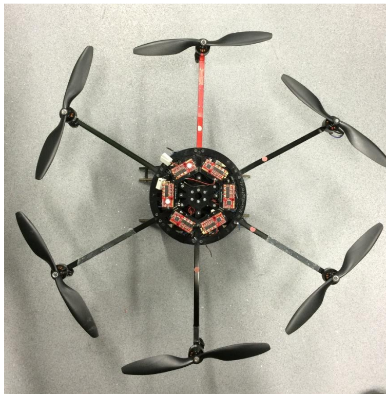
Figure 4.1 - MikroKopter multi-rotor platform from above with the red arm indicating the nominal forward direction.
