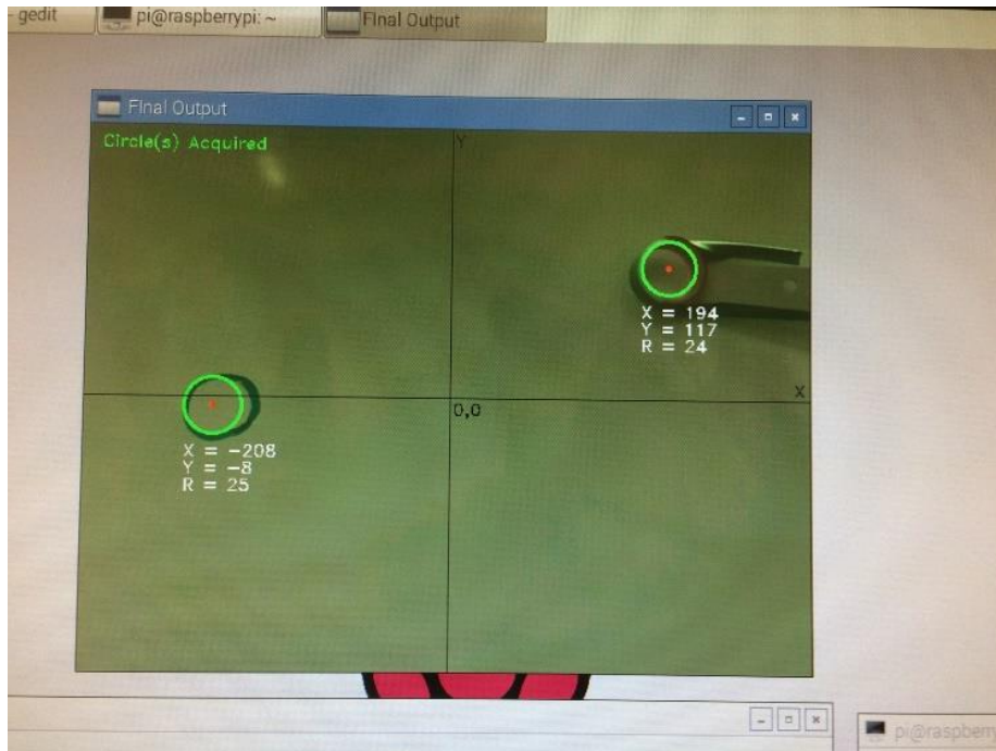
Figure 6.8 - Screenshot of the image from PiCamera detecting two drawn circles.
