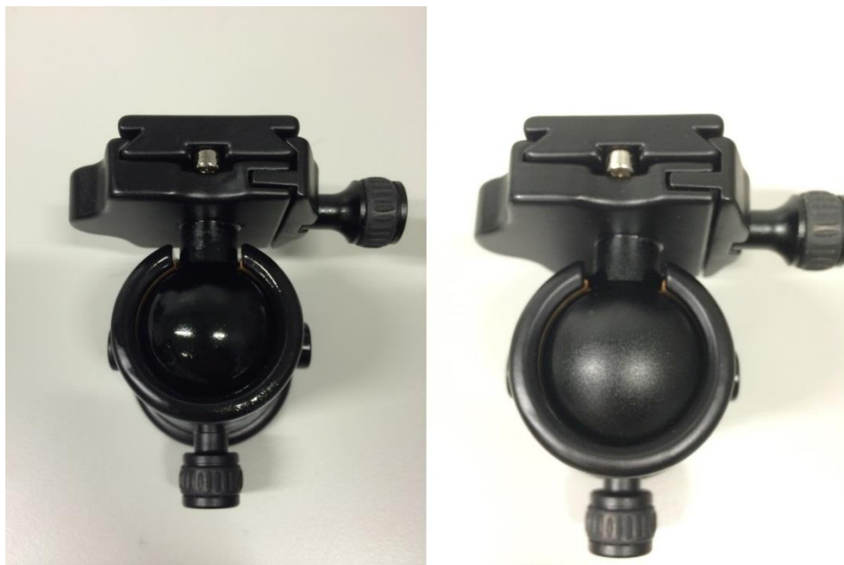
Figure 4.23 - The gimbal ball joint which shows the ball lubricated and unlubricated.
