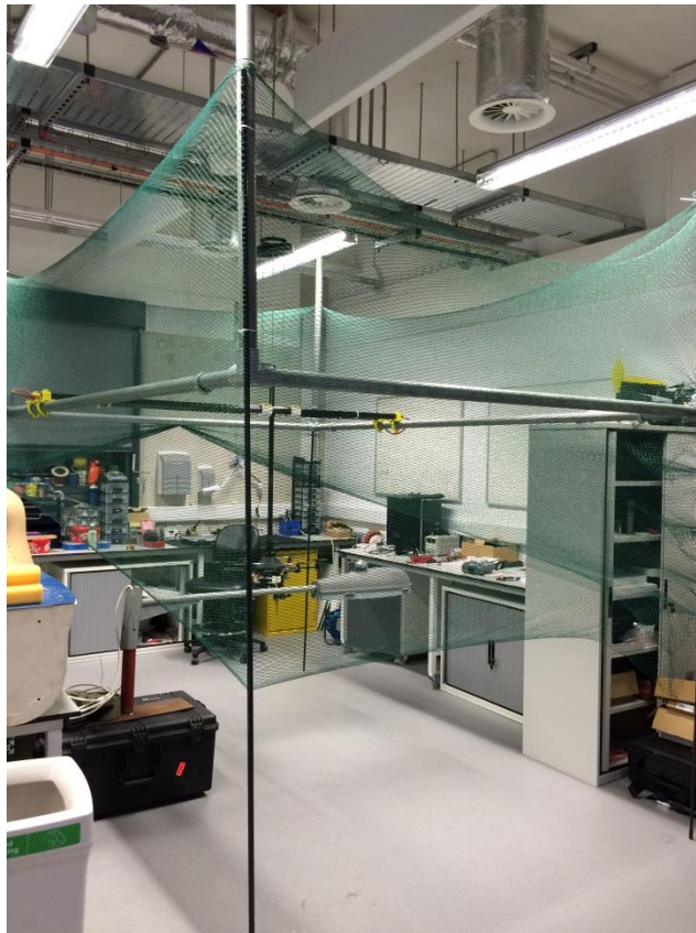
Figure 4.24 - Final finished test-rig with green netting, attached UAV and projection bracket set up.
