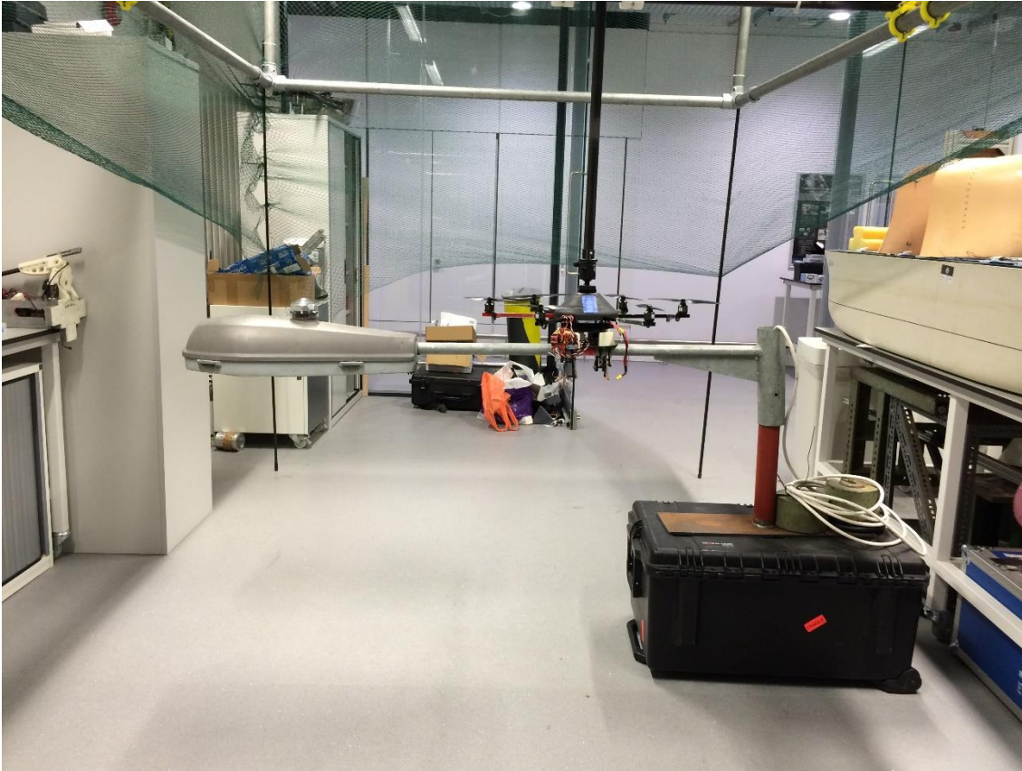
Figure 6.12 - Cluttered environment allowing for prop-wash to cause disturbances.
