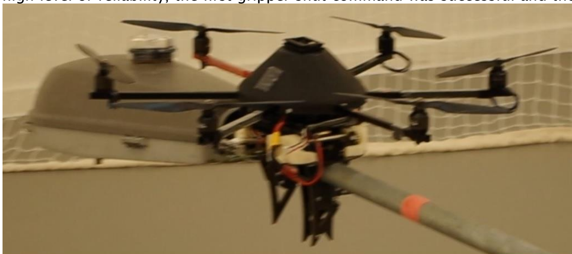
Figure 6.23 - The final perched position of the UAV with the gripper shut tight.
