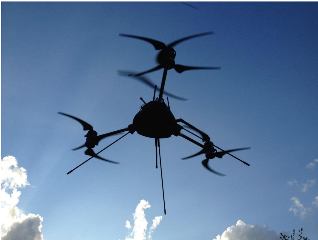
Figure 1.3 - HALO UAV at the competition in GA. Fort Stewart. HALO's specially designed legs gave it the ability to perch on rooftops simply by descending down until it wedged itself onto the angle of the roof.
