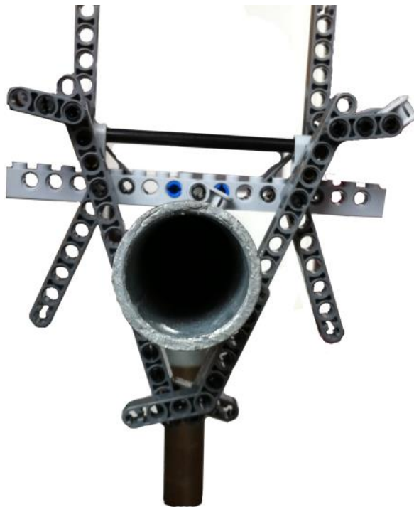
Figure 3.14 - The Claw design model gripping the projection bracket (a more detailed Lego prototype).
