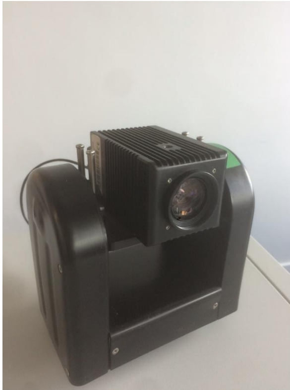
Figure 6.1 - Gimballed camera unit from Bradley Engineering used for visual tracking.
