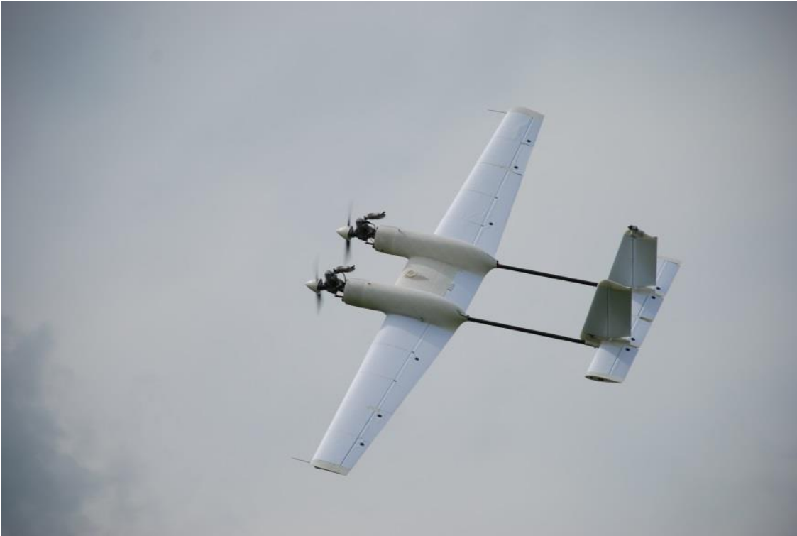
Figure 2.1 - 'Spotter' a fixed wing UAV with 4 m wingspan and twin engine and twin autopilot design which allows for redundancy.
