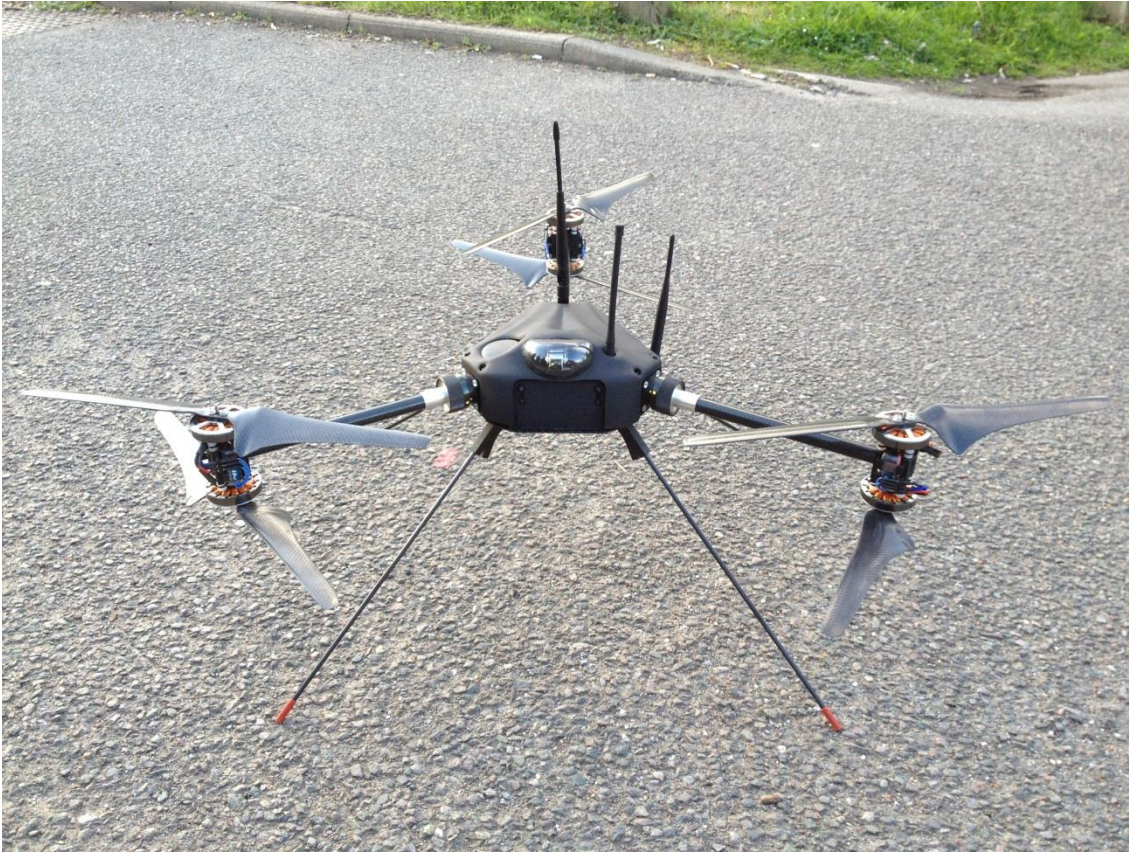
Figure 2.3 - HALO UAV with three arms and each arm containing a co-axial motor and propeller configuration.
