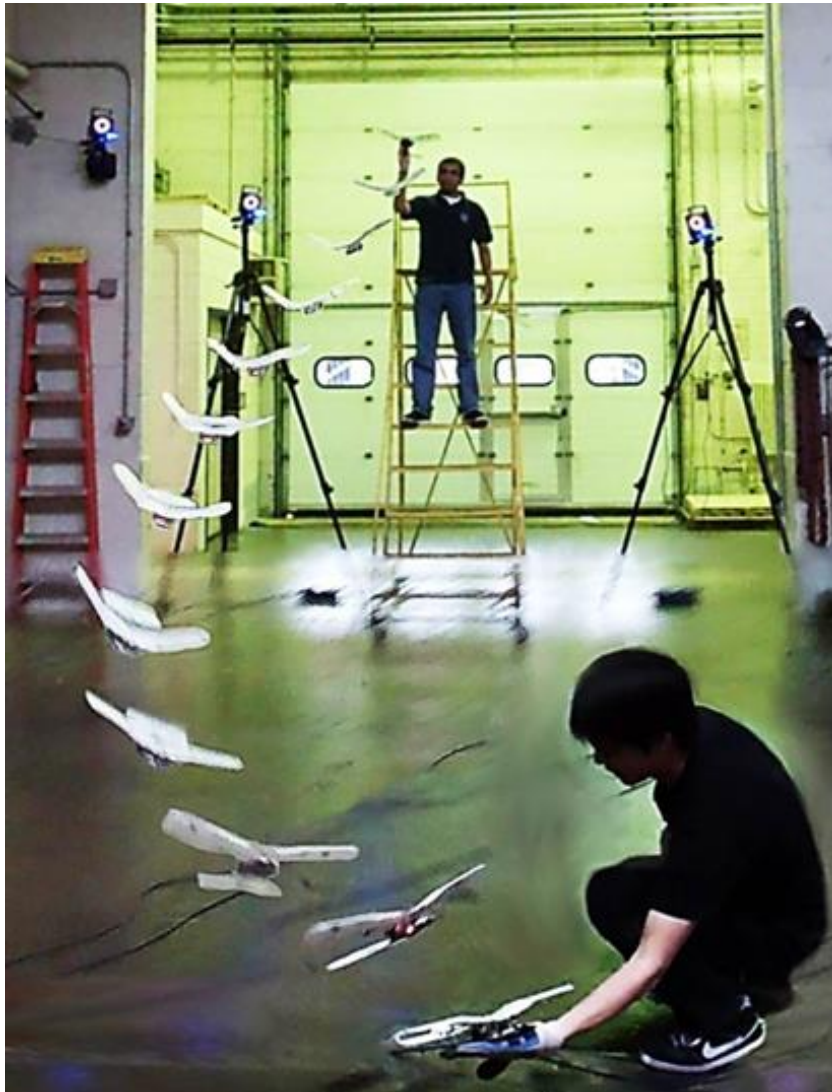
Figure 2.7 - Sequential image of the flapping wing system being launched at one end and caught at another (Used with permission of Paranjape).
