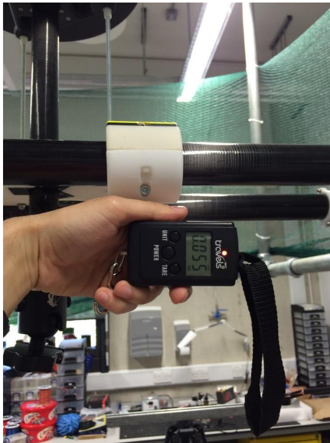
Figure 4.22 - Image of the XZ runner being pulled using a strain gauge.
