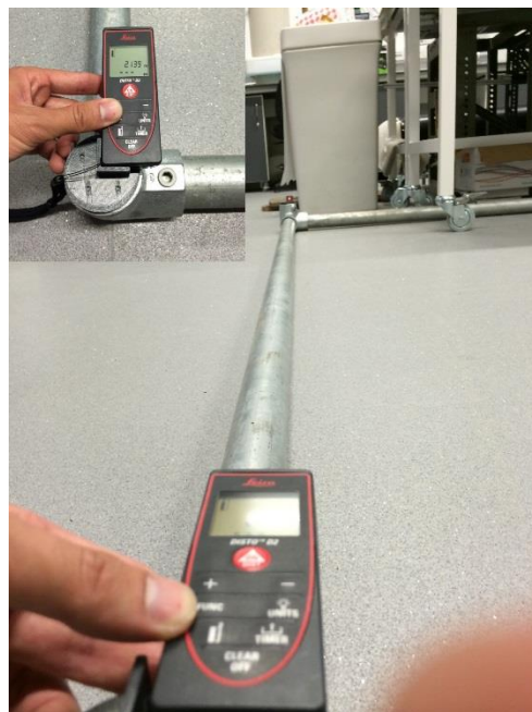
Figure 4.18 - Test-rig corner point measuring tool allowed for the laser range measuring device to measure from the centre of the vertical axis of the 3 elbow corner units.
