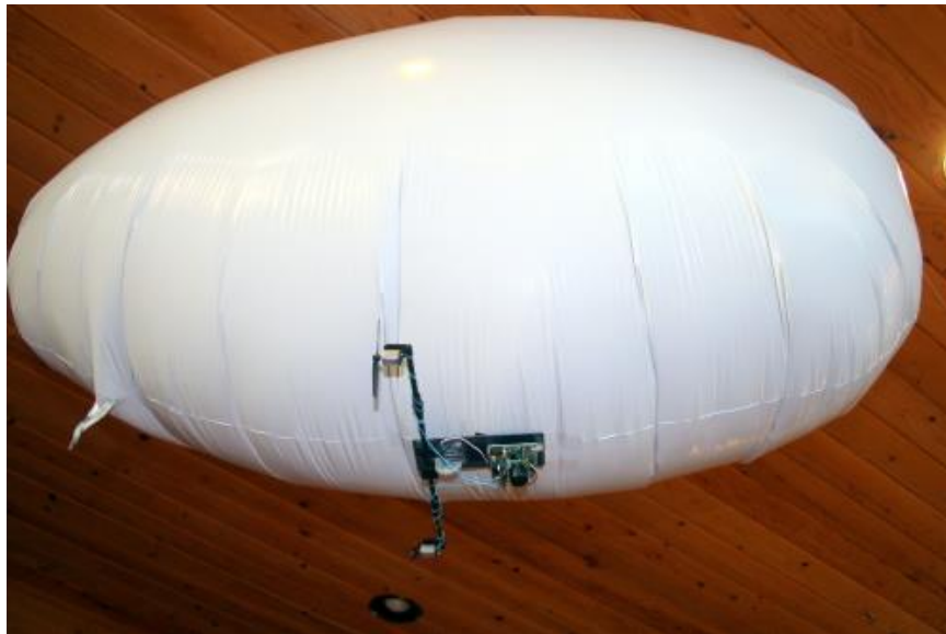
Figure 2.4 - BlimpDuino which has the control system attached below (Used with permission of Chris Anderson).
