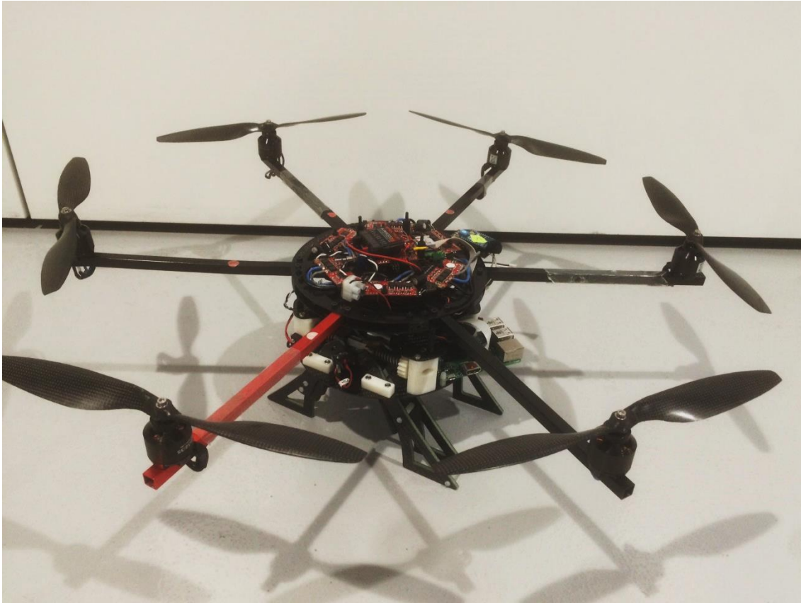
Figure 6.21 - The final UAV with perching element attached and ready to be tested.
