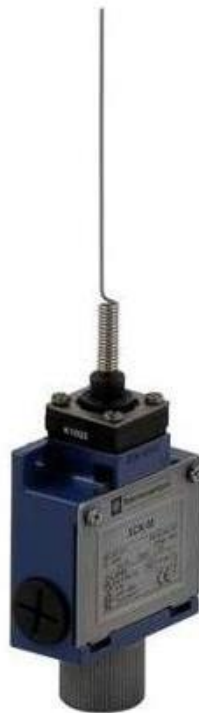
Figure 6.4 - Whisker Switch with spring base to ensure contact returns to same position.
