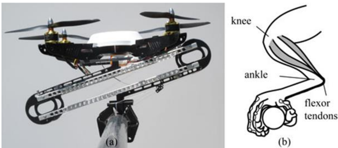
Figure 2.18 - Passive perching system which takes its inspiration from the gripping system of a Sorrow bird (Used with permission of Doyle).
