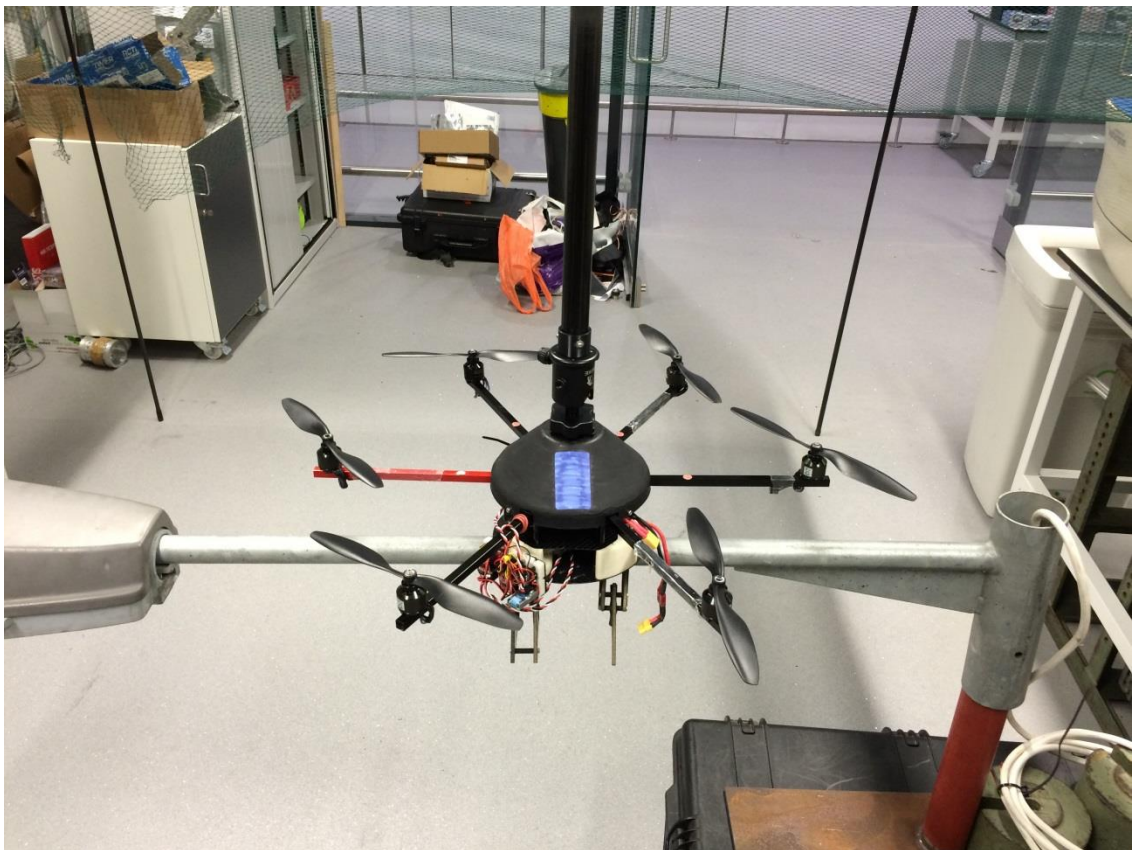
Figure 4.25 - The UAV was flown manually to quickly determine the movements of the UAV and the free movement of the test-rig.
