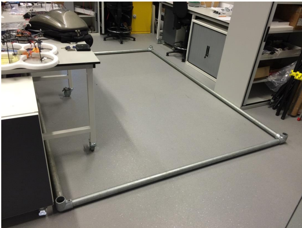
Figure 4.14 - Test-rig set up on floor and levelled out using shims to ensure accurate levelling. Digital level was used to take measurements.
