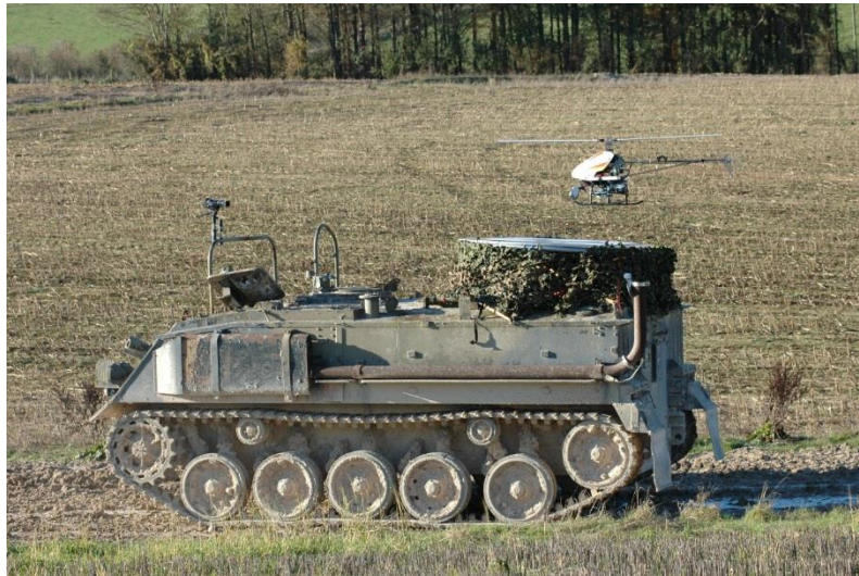
Figure 2.16 - Image of helicopter with the autoland system being tested on moving Armoured personnel carrier (APC) (Image courtesy Chemring Technology Solutions).
