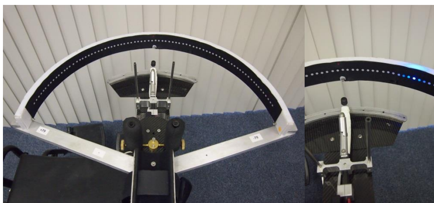
Figure 5.12 Black paper on a white curve of the redesigned wrist rig
