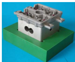
n) Dismountable real workpiece-like reference object, PTB, BAM [72]
