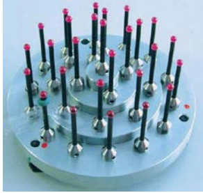
d) 27 ruby spheres, Zeiss [65]
