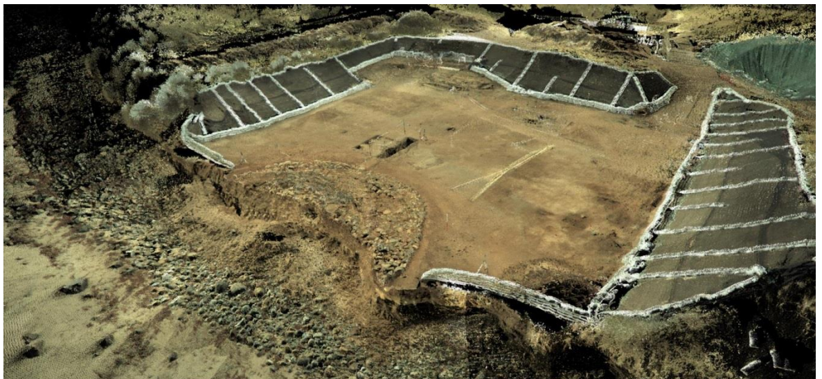
Figure 36 – Results of the terrestrial laser scanning survey of the site at Low Hauxley (see Chapter 8 below), with RGB colour values taken from the internal camera mapped over the point cloud.
