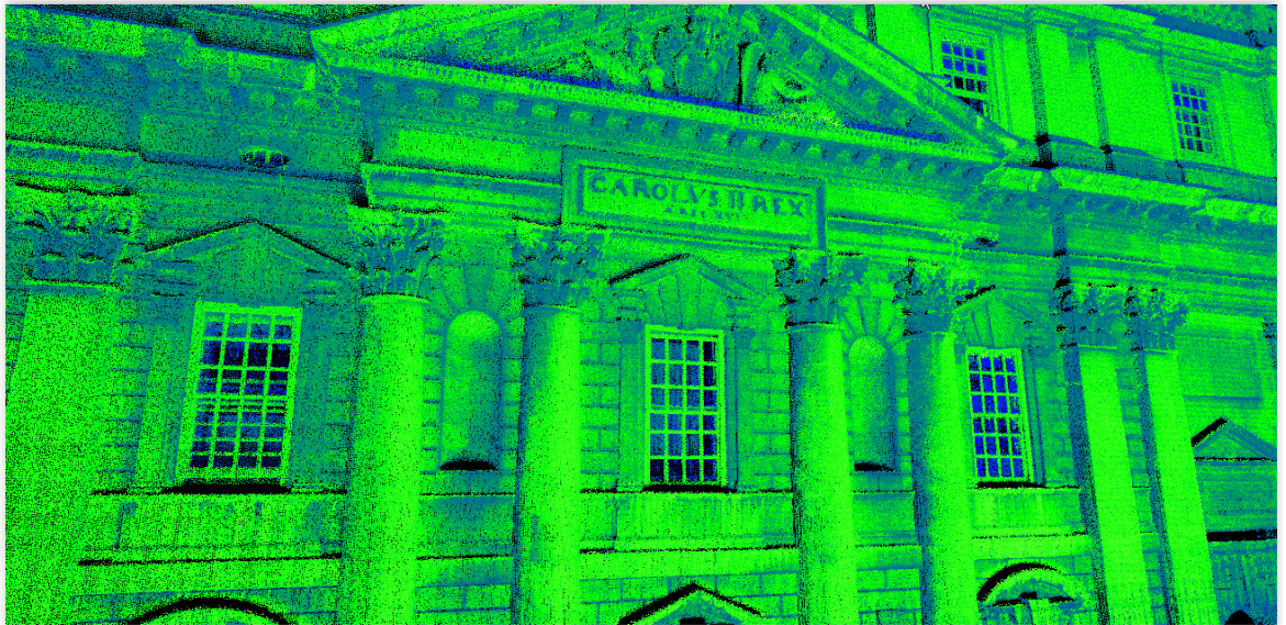
Figure 35 – Point cloud created from the terrestrial laser scanning survey of the Old Royal Naval College in Greenwich. Each point represents an x, y, z measurement, with the colours representing the strength of intensity returns reflecting from differing surface materials.
