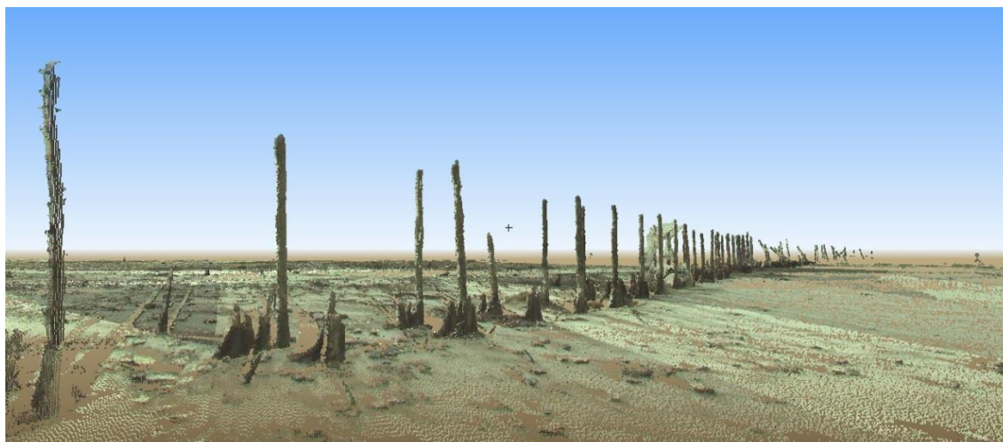
Figure 47 – Results of the terrestrial laser scanning survey of the structure at Aust, Severn Estuary. The RGB values from the internal camera have been draped over the point cloud to create a realistic image of the structure.
