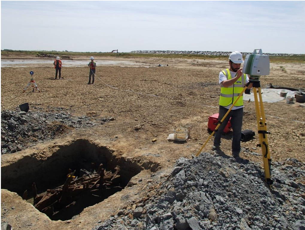
Figure 87 – Terrestrial laser scanning of trench 2 of the linear wattle-built structure at Medmerry
