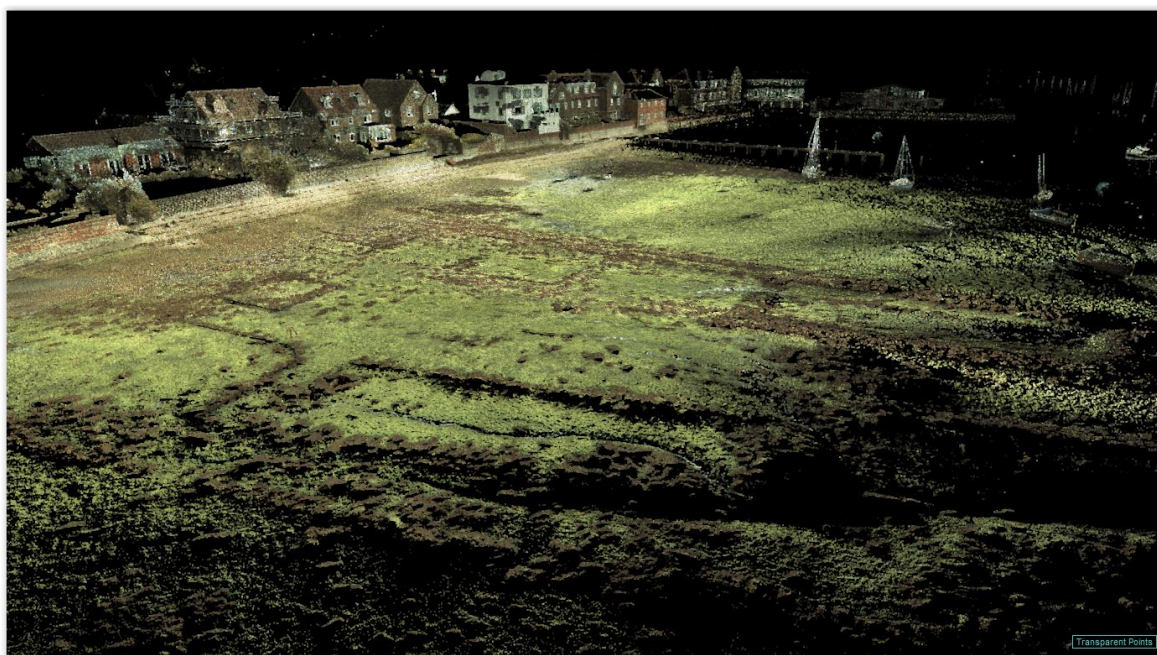
Figure 78 – Screenshot showing the results of the terrestrial laser scanning survey on the foreshore at Emsworth viewed from the west
