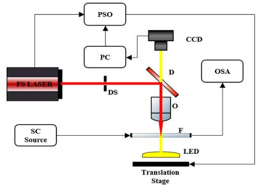
Figure 1 – Schematic diagram of femtosecond writing set up. **O**-Objective, **D**-Dichroic mirror, **F**-Fibre, **DS**-Diffraction slit, **PSO**-Synchronisation Controller, **LED** – Light Emitting Diode.
