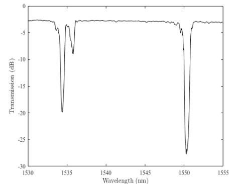
Figure 3 – T transmission spectra of the grating inscribed at  $\lambda_B \sim 1550$  nm. Secondary resonances were observed at  $\lambda_B \sim 1534$  nm and 1536 nm due to higher modes.
