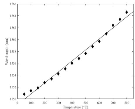
Figure 4 – Thermal testing results showing shift in the Bragg wavelength against temperature. Regression deduced a sensitivity of  $\sim 18.5$  pm/°C.
