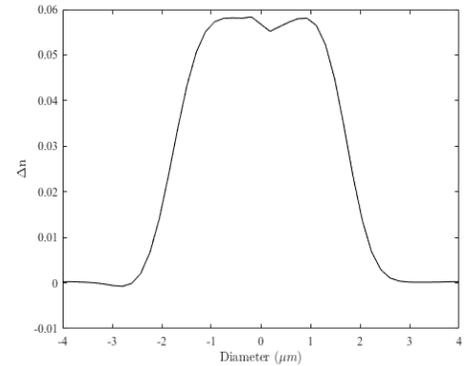
Figure 2 – Refractive index profile of the high concentration germanium fibre core with NA = 0.41.
