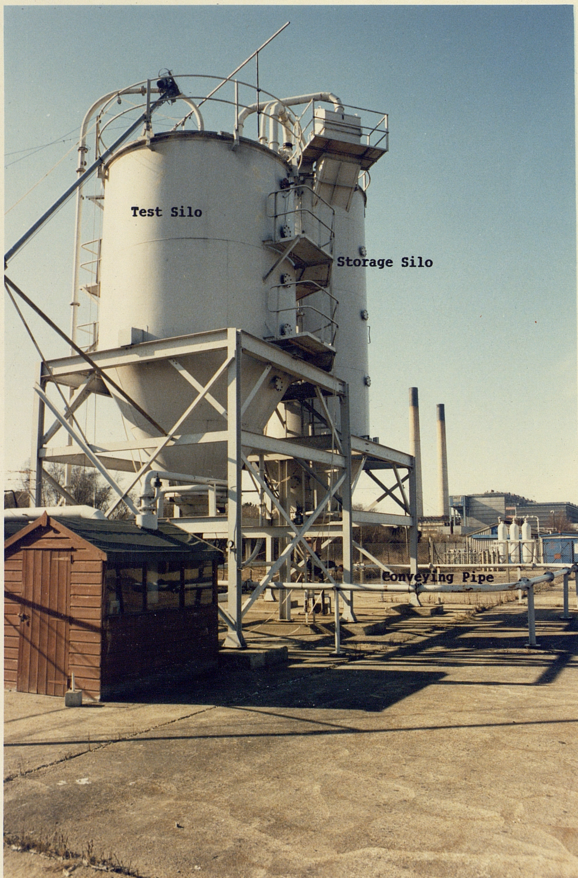
Figure 2.1b Industrial Scale Experimental Rig (Marchwood Silo Rig)
