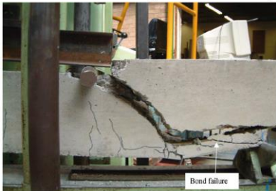
Figure 1. (a) Catastrophic failures noted in concrete beams reinforced with FRP bars [5] (b) Applied load–midspan deflection relationships of concrete beams reinforced with GFRP and CFRP bars [6]
