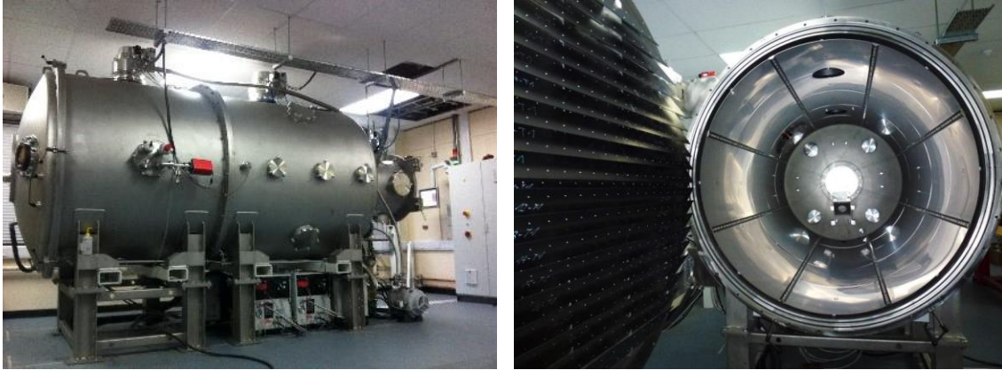
Figure 8. Overview of the David Fearn Electric Propulsion Laboratory at the University of Southampton (left) and the 4m long by 2m diameter test chamber section (right).
