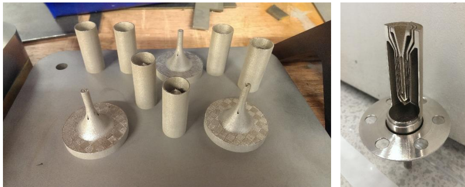
Figure 6. Thruster and Thruster Inflow as-printed components on the Concept Laser M2 Cusing base plate (left) and the two components assembled with a polished Thruster section.
