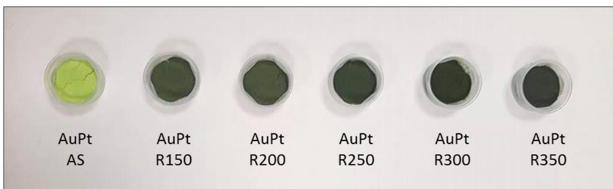
Figure 3.14: Photograph of the as-synthesised and reduced AuPt/CuClP materials; reduced materials have been activated at 150^\circ\text{C} (R150), 200^\circ\text{C} (R200), 250^\circ\text{C} (R250), 300^\circ\text{C} (R300), and 350^\circ\text{C} (R350).
