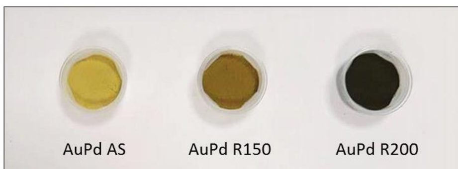
Figure 3.22: Photograph of the as-synthesised and reduced AuPd/CuClP materials; reduced materials have been activated at 150 °C (R150) and 200 °C (R200).
