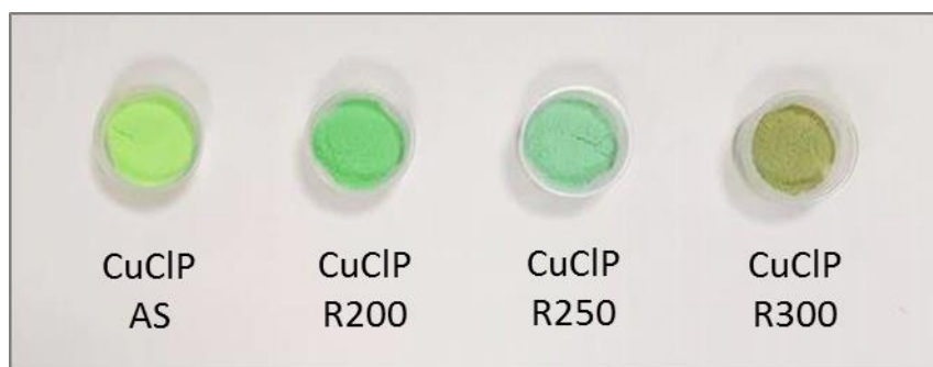
Figure 3.4: Photograph of the as-synthesised and reduced CuCIP materials; reduced materials have been activated at 200 °C (R200), 250 °C (R250) and 300 °C (R300).
