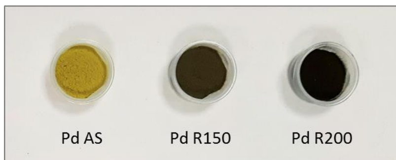
Figure 3.10: Photograph of the as-synthesised and reduced Pd/CuClP materials; reduced materials have been activated at 150^\circ\text{C} (R150) and 200^\circ\text{C} (R200).
