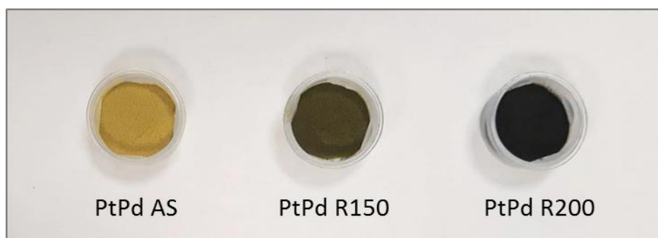
Figure 3.18: Photograph of the as-synthesised and reduced PtPd/CuClP materials; reduced materials have been activated at 150 °C (R150) and 200 °C (R200).
