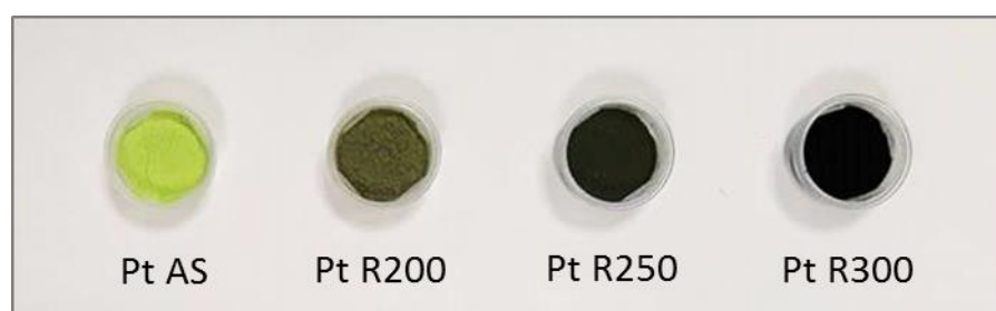
Figure 3.8: Photograph of the as-synthesised and reduced Pt/CuCIP materials; reduced materials have been activated at 200 °C (R200), 250 °C (R250) and 300 °C (R300).
