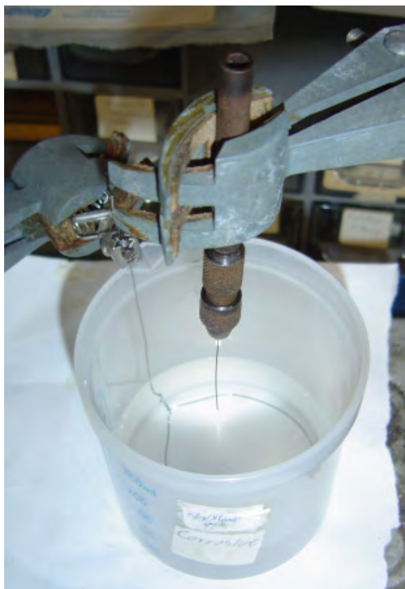
Figure 2.16: Showing the plastic beaker and smaller stainless ring used for DC etching.
