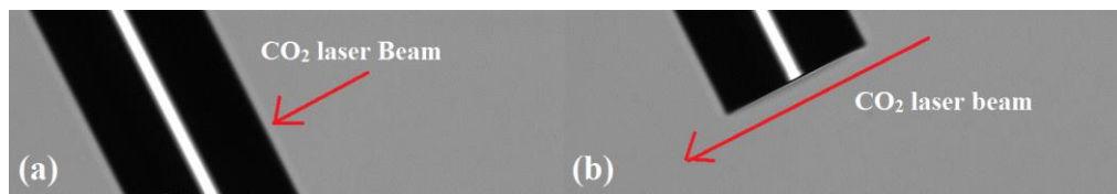
Figure 3.20: a) Only stripping of the fibre is required as a preparation process prior to cleaving. b) Resulting end-face after a CO 2 'cleaving' process [18].
