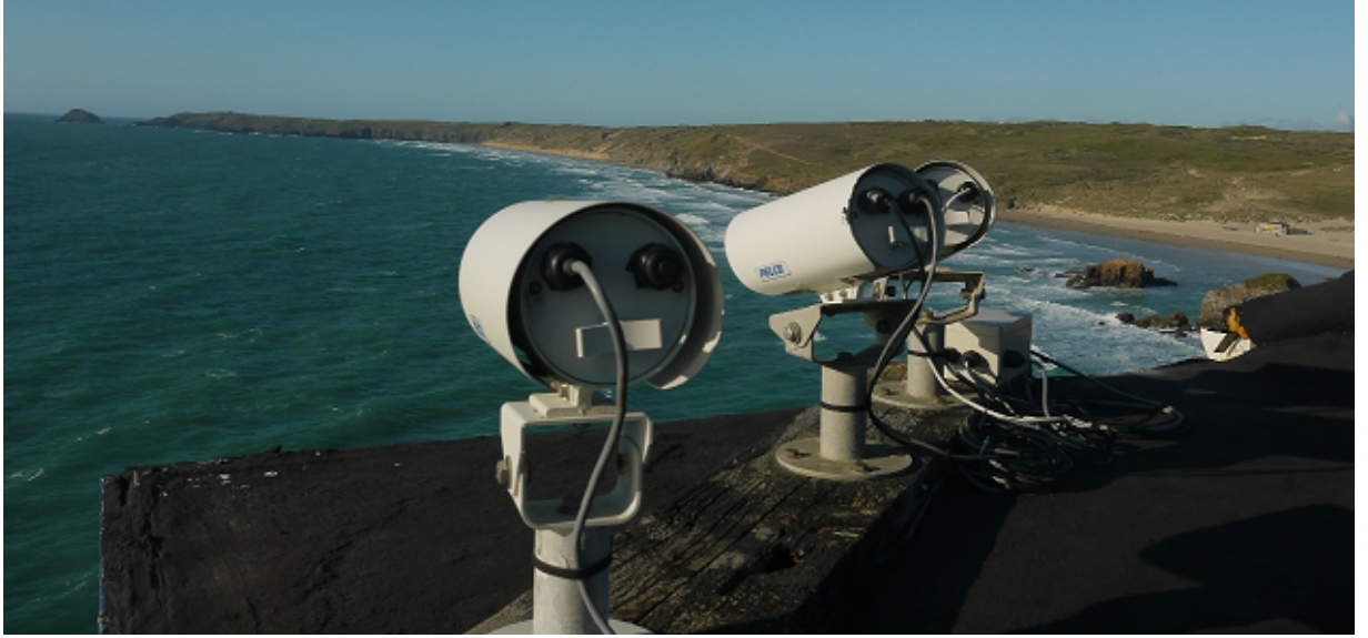
Figure 2.1: The three-camera monitoring system installed at Droskyn Point to monitor Perranporth. Picture taken at high tide, with cameras orientated to capture low tide intertidal beach area. Photo credit: S Pitman.
