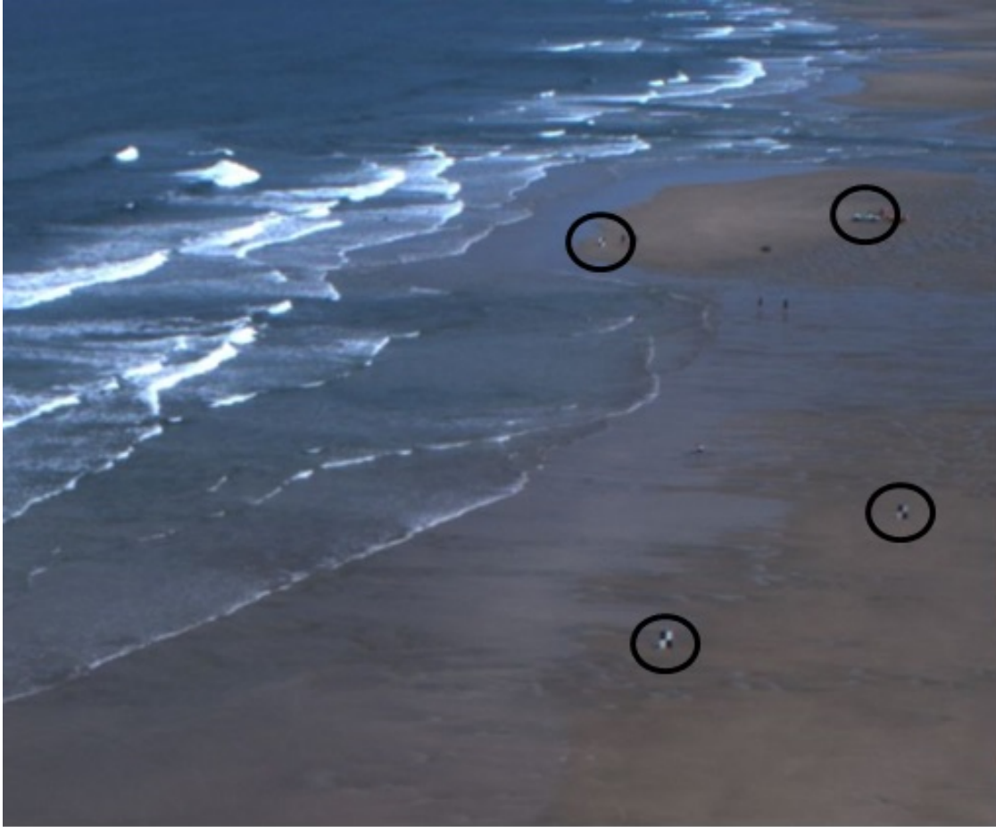
Figure 2.4: Example use of temporary GCPs (when no permanent features are visible in the image) at Perranporth, U.K. This image depicts checker boards placed on the beach (black circles), providing easily identifiable static positions in the image. Additionally, the static RNLI truck has also been used as an extra GCP. Photo extract from Argus archive.
