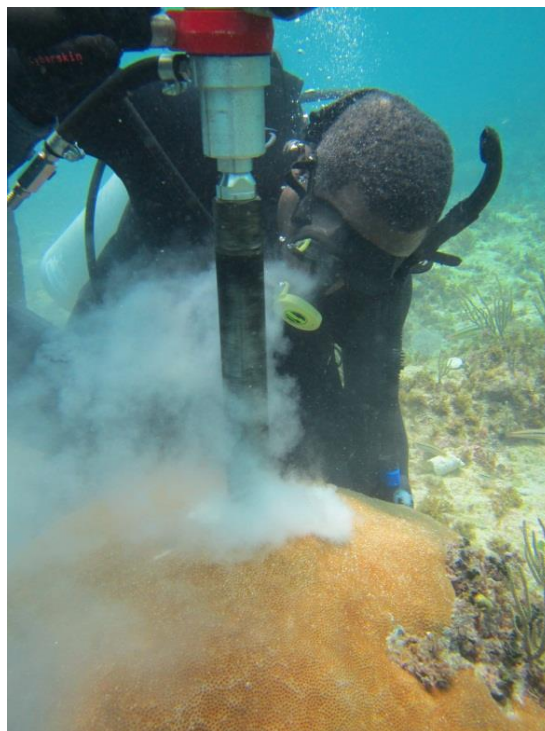
Figure 2-2. Dr Karl Castillo coring a Siderastrea siderea colony using a pneumatic air drill with a hollow extension rod and wet diamond core bit. Credit: Dr Karl Castillo.
