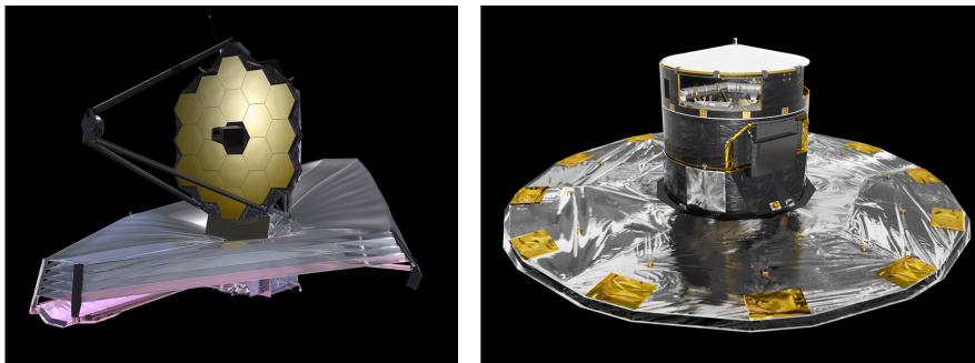
Figure 5.20: Thermal shield used for the James Webb Space Telescope (left image) [14] and for Gaia (right image) (courtesy of ESA).
