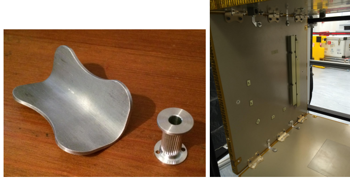
Figure 4.27: Metallic connectors between the panels, inserts and LHP.
