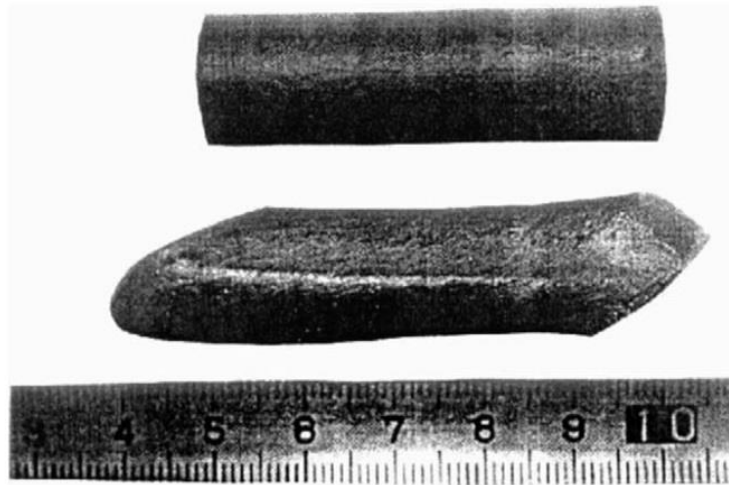
Figure 2.27 Tungsten billet processed by ECAP using Route B C and \phi = 110^\circ for 8 passes [78].
