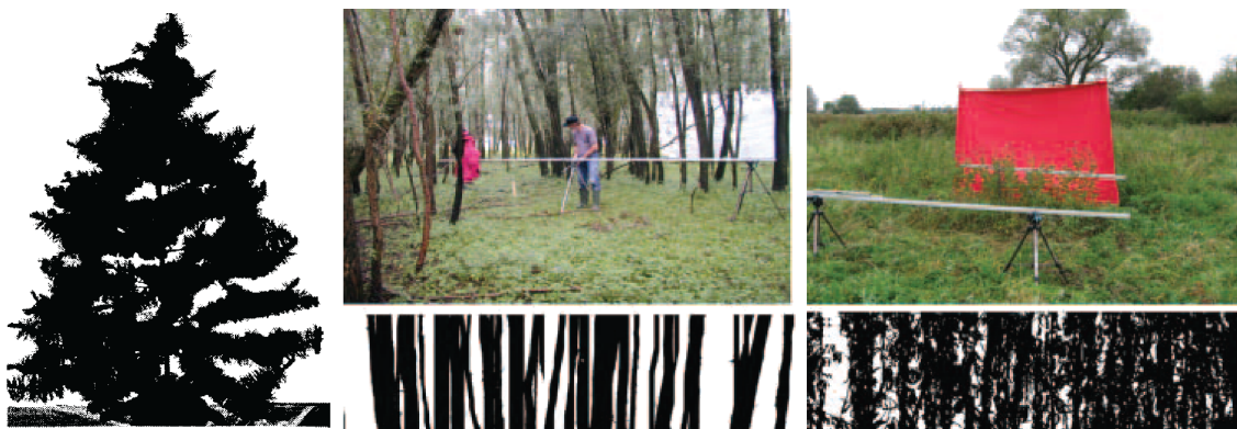
FIGURE 4.3: Binary image of artificial scots pine taken in front of white backdrop. The amount of white pixels within the plant area provides a 2D plant porosity estimate (left) (Source: Figure 3 from Grant and Nickling, 1998). Collection of parallel photography images against a high contrast backdrop for tree (middle) and herbaceous (right) vegetation of a floodplain, and derived binary images (Source: Figure 2 from Straatsma et al., 2008).
