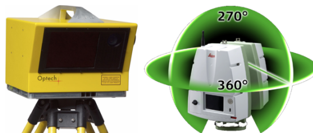
FIGURE 4.5: Examples of different types of TLS instruments. Optech ILRIS 3D, window-like system with field of view 40^\circ \times 40^\circ (left); Leica ScanStation C10 with rotating polygonal mirror with field of view 360^\circ \times 270^\circ (right).
