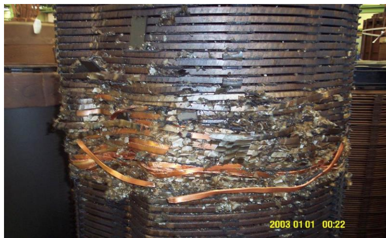
Figure 2.1.2 A transformer winding that has suffered catastrophic failure [26]
