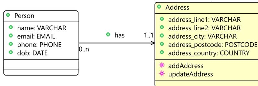
Figure 6: An example of an outer entity
