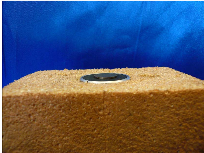
(a) Disc magnet resting on a superconducting pellet in the resistive state.
