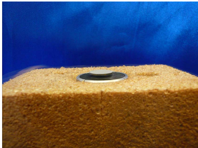
(b) Disc magnet levitating above a superconducting pellet in the superconducting state, levitating due to the complete expulsion of the magnetic field, known as the Meissner effect.
