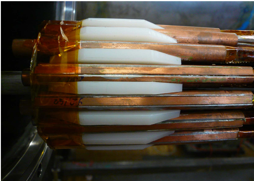
Figure 2.11: Assembled intra-pair joints at the bottom of the cable. Notable features include copper joint lids and PTFE holder/separator.
