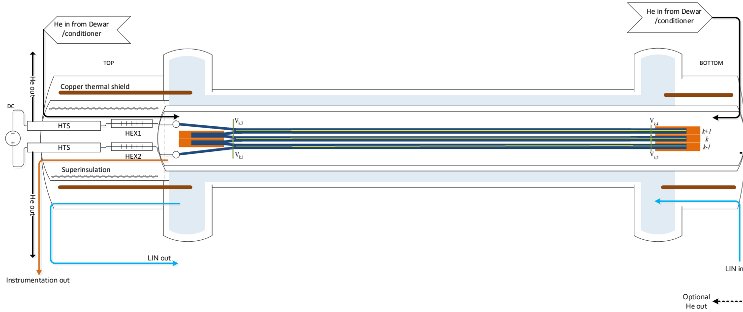
Figure 2.1: Schematic of 5 m Nexans semi-flexible cryostat at the University of Southampton showing all entry/exit ports apart from vacuum ports. Vertical dashed line represents flange at which cryostat opens for loading and connection of sample. Superconducting cable to be tested represented by schematic from [44]. HEX = Heat exchanger, LIN = Liquid Nitrogen, other abbreviations as in Glossary.
