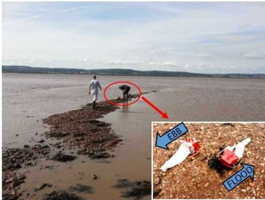
Figure 4.16 A pair of Helley-Smith bedload sediment traps are set up on the crest of dune (red circle). The inset shows the traps are facing the flood and ebb directions in order to sample bedload sediment being transported in opposing directions.
