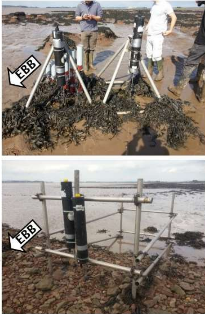
Figure 4.9 Current meters set in different height in the dune field. (Top) Aluminium tripods were used to install current meters above the bedrock close to dune crest in the early deployment (2013); the left-hand meter measured flow at 15 cm above the bed and the right-hand meter measured flow at 40 cm above the bedform; (Bottom) A scaffold was set on the dune crest in 2014 to replace the tripods.
