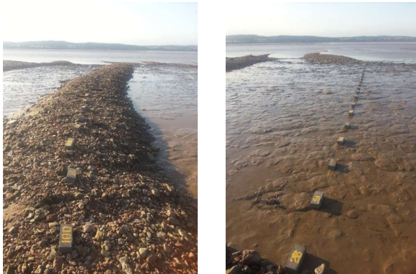
Figure 4.22 Two rows of bricks were aligned on the crest (left) and trough (right) from onshore towards the river channel. Each row consists of 25 bricks individually identified by painted numbers.
