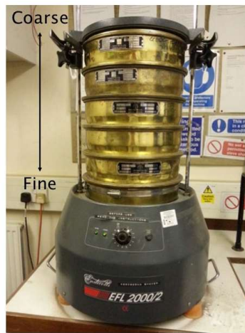
Figure 4.19 Sieve shaker: a machine used in sorting dried sediment sample into classes. Sieves are stacked regarding to aperture size; the coarsest sieve is on the top while the finest is at the bottom of the stack.
