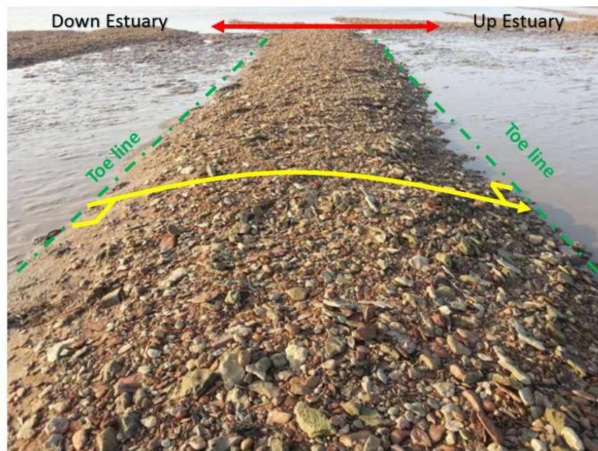
Figure 4.7 Direction of cross-section survey. The measurement starts from down estuary toe to up estuary toe for every 50 cm. The start and end points are perpendicular to toe lines.
