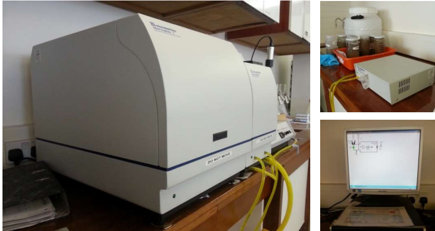
Figure 4.20 Saturn DigiSizer unit (Model: II 5205 V1.02): the machine fine particle sizing instrument
