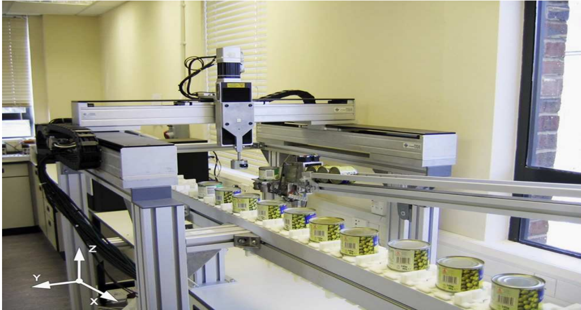
Figure 6.1: The gantry robot with the three axes marked.
