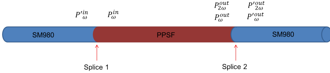
FIGURE 5.11: Schematic of the typical all-fibre nonlinear device for frequency doubling realized by splicing the PPSF with two pieces of SM980 fibre. The reason of the presence of these two “buffers” is mainly related to the fact that it was experimentally observed that splicing the PPSF with the SM980 fibre instead of with the SMF28 fibre allows for reducing the insertion losses because of a better matching of the two core’s sizes spliced together. The splice losses between the SM980 and the SMF28 fibres are assumed negligible.
