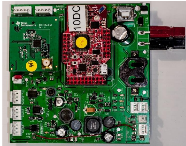
Figure 20: Photograph of the MS1 sensor node design with attached Zolertia Z1 and CC1120 radio board.
