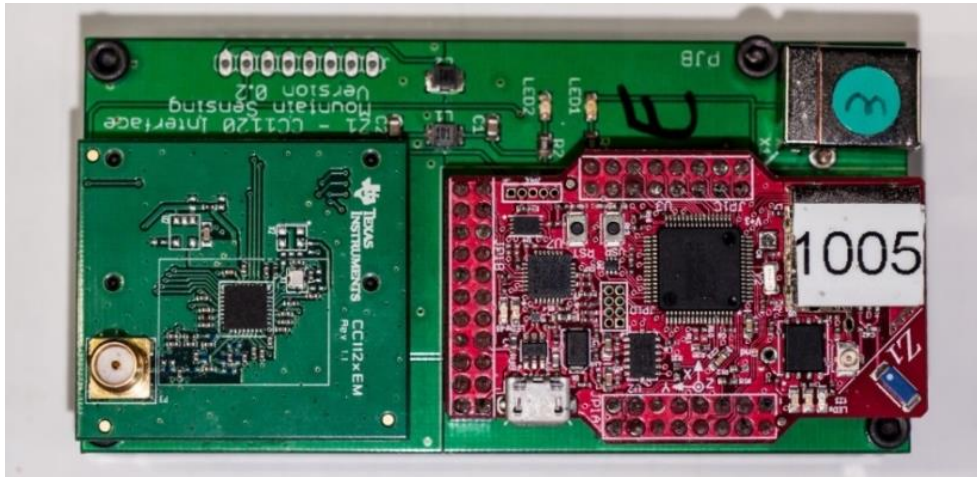
Figure 11: Test hardware consisting of a CC1120EM (left), Zolertia Z1 (right) and a bespoke interface board.
