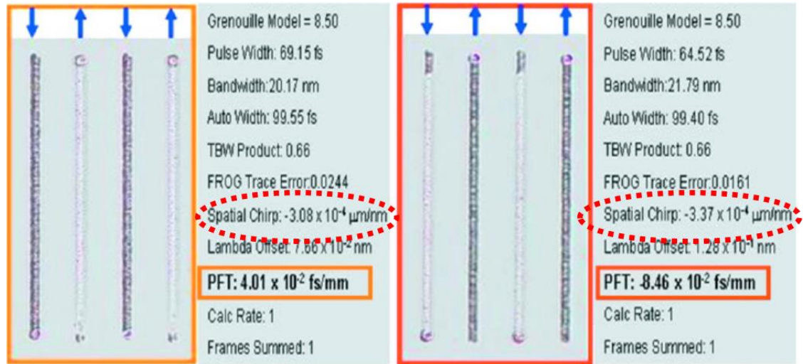
Figure 8.6: The quill-effect was thought to have flipped due to a change in sign of the TC. However, the PFT doubles in magnitude while the SC stayed constant. Upon further review, the SC value is unphysical, thus re-opening the discussion on what causes the quill-writing effect. Image source: Yang et al. [5]
